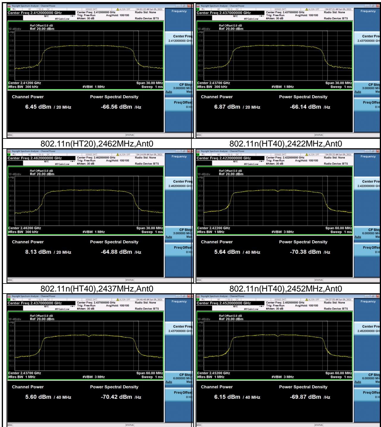
**TEST REPORT****4. Power spectrum density****4.1 Test Data**
