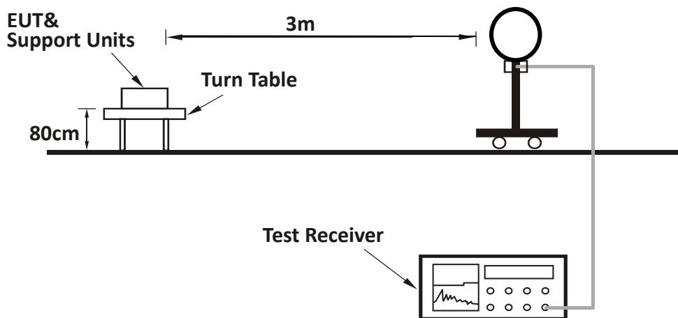
For Radiated emission 30MHz to 1GHz:
