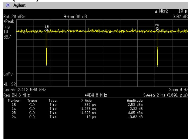
$$\text{Duty Cycle} = T_{\text{on}} / (T_{\text{on}} + T_{\text{off}}) = 1276[\text{us}] / (1276[\text{us}] + 8[\text{us}]) = 99.22[\%]$$
