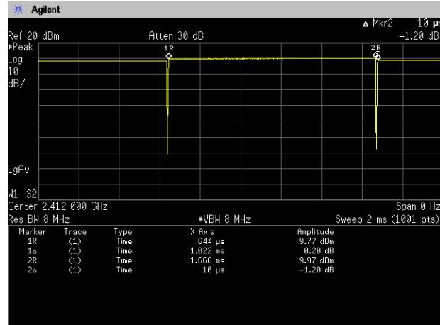
$$\text{Duty Cycle} = T_{\text{on}} / (T_{\text{on}} + T_{\text{off}}) = 1022[\text{us}] / (1022[\text{us}] + 10[\text{us}]) = 99.03[\%]$$
