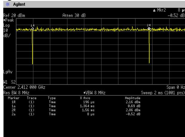
$$\text{Duty Cycle} = T_{\text{on}} / (T_{\text{on}} + T_{\text{off}}) = 1364[\text{us}] / (1364[\text{us}] + 8[\text{us}]) = 99.42[\%]$$
