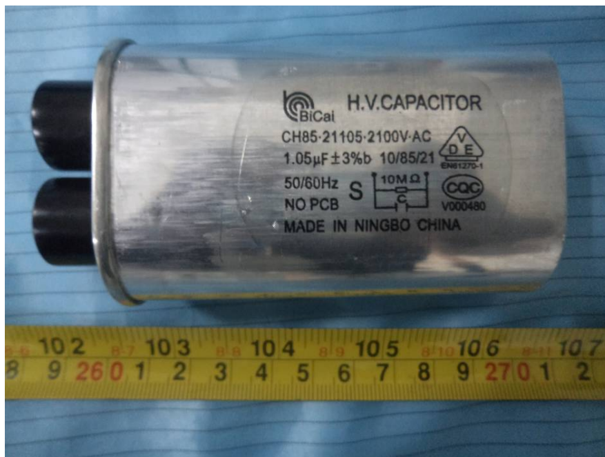
EUT – H.V. Capacitor View
