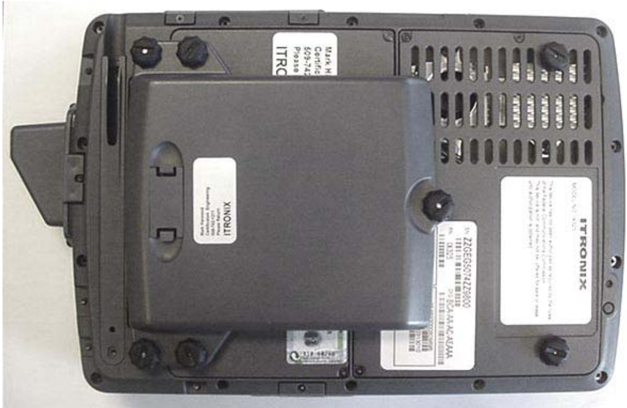
DUT with External Second Li-ion Battery 11.1 V, 3600 mAh (Model: T8S-E)
