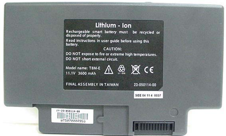
Internal Li-ion Battery 11.1 V, 3600 mAh (Model: T8M-E)
