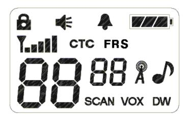
Key lock indicator: Indicates that the key lock function is in use Beep ON/OFF indicator: Appears while key tone is in use. Battery indicator: Indicates the battery status.
