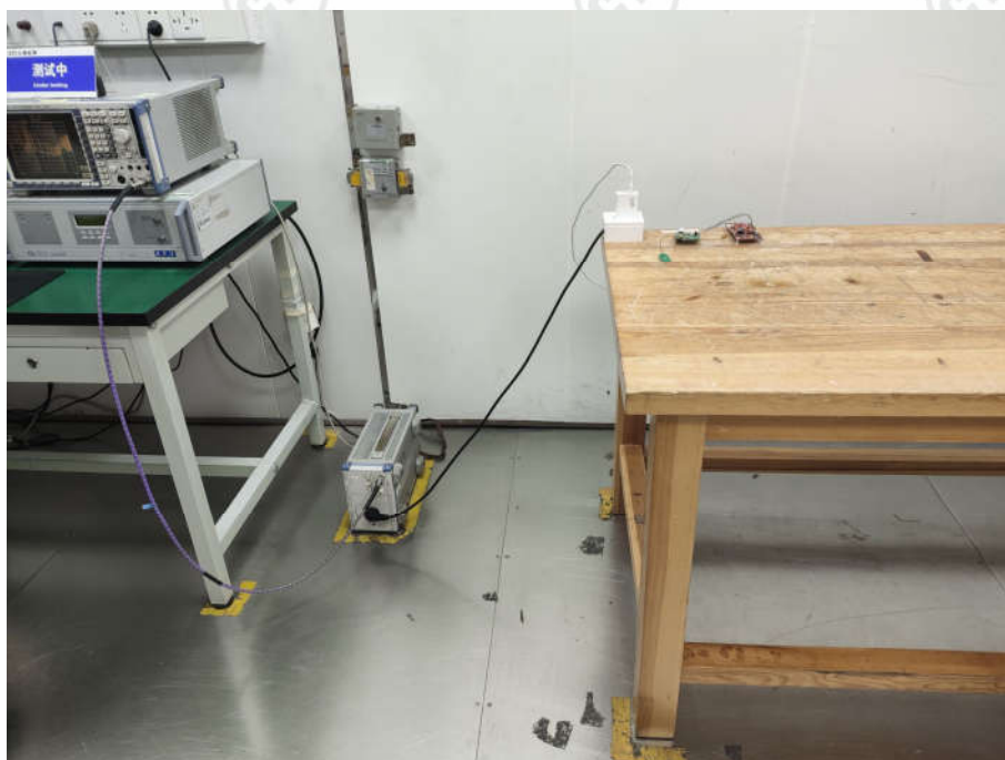
Conducted Emissions Test Setup
