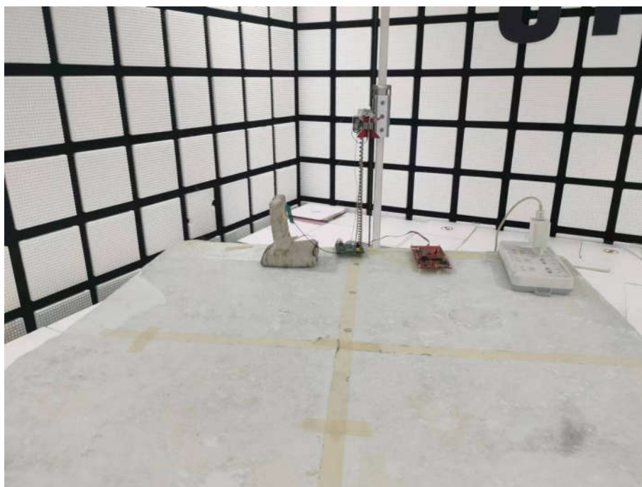
Radiated spurious emission Test Setup-2(Above 1GHz)
