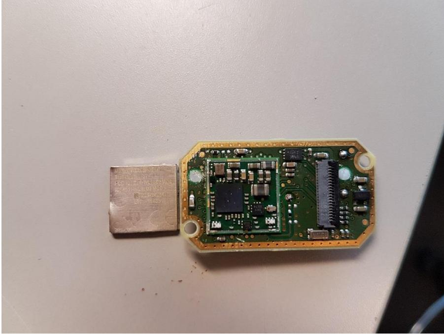
*Figure 3 Radio module without cover.*
