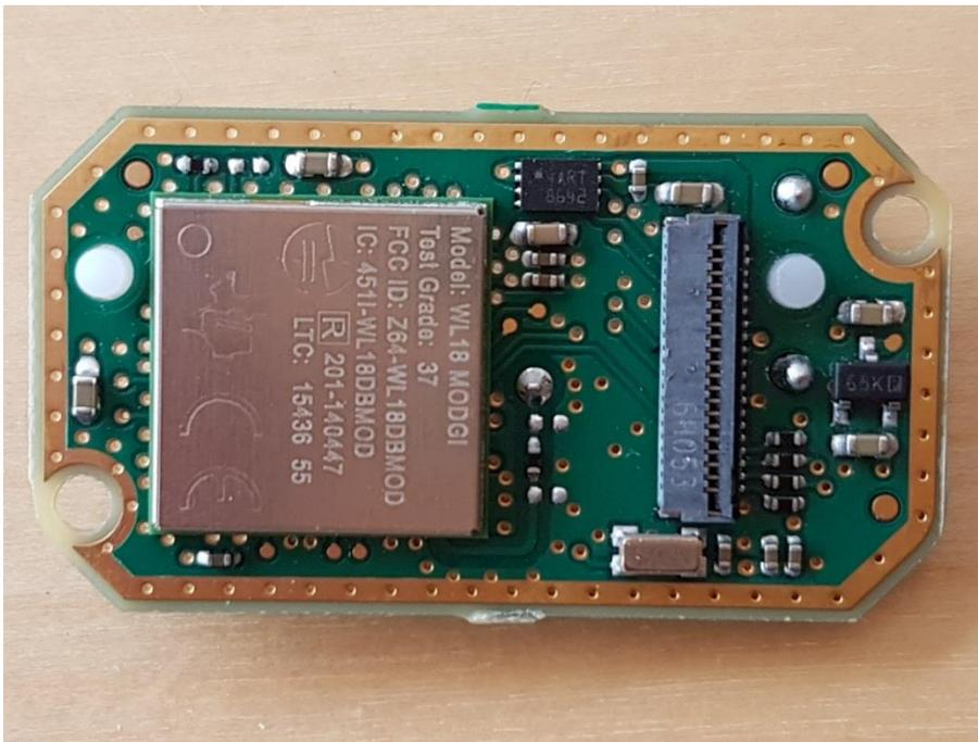
Figure 2 EVBW2 Radio board
