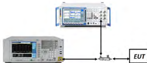
Figure 7-2. Test Instrument & Measurement Setup
