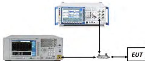
Figure 7-4. Test Instrument & Measurement Setup
