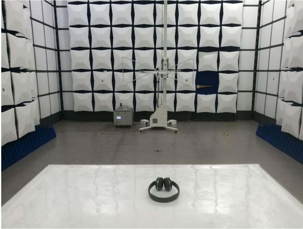
FCC RADIATED EMISSION TEST SETUP
