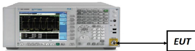
Figure 7-2. Test Instrument & Measurement Setup
