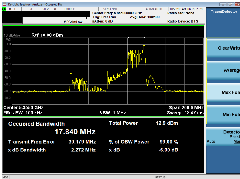
Plot 7-51. 6dB Bandwidth Plot MIMO ANT1 (80MHz BW 802.11ax – 26 Tones (UNII Band 3/4) – Ch. 171)
