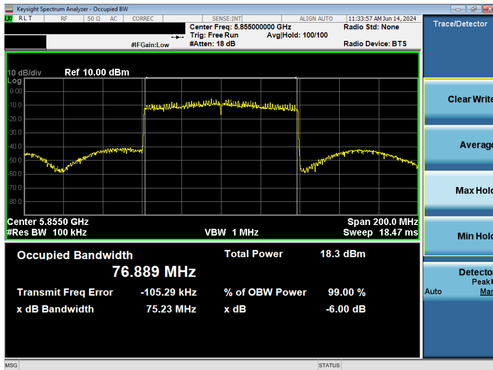
Plot 7-58. 6dB Bandwidth Plot MIMO ANT1 (80MHz BW 802.11ax – 996 Tones (UNII Band 3/4) – Ch. 171)
