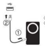
①Connect the USB-C to the port on the side of Ascend Charge.
