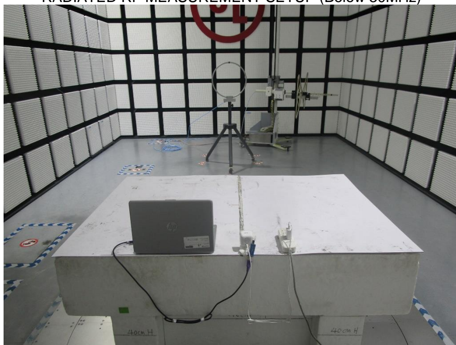
RADIATED RF MEASUREMENT SETUP (Below 30MHz)
