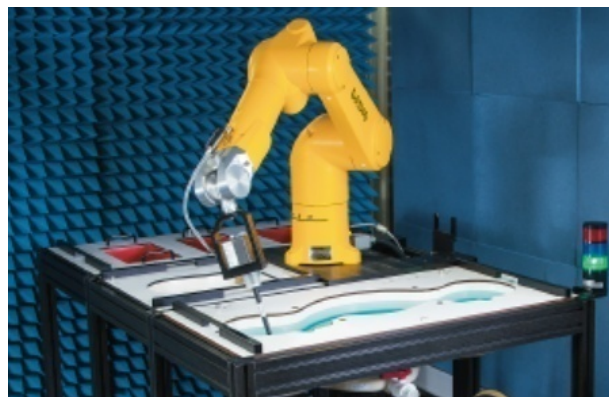
Fig 6.5 Photo of DASY5
