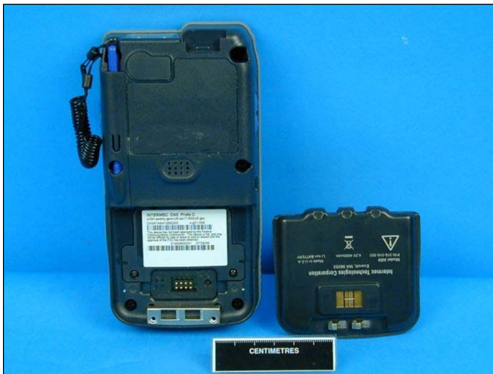
Figure 54: Rear View of the Intermec CN3 – Battery removed.
