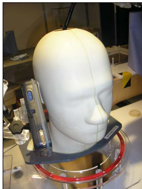
Figure 45. Positional photograph of the Intermec CN3 Right Hand Cheek 15° Position
