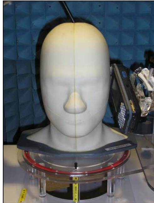
Figure 43. Positional photograph of the Intermec CN3 Left Hand Cheek 15° Position
