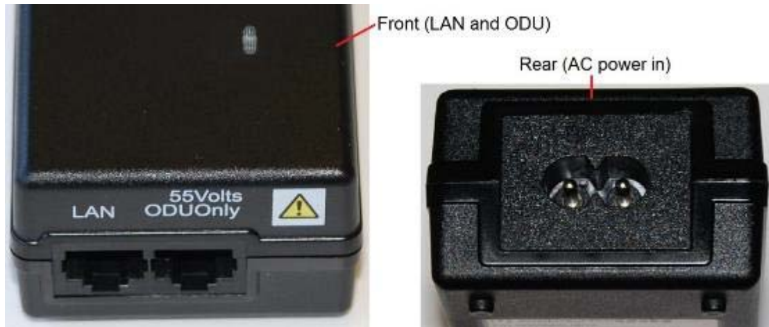
Figure 15 AC Power Injector interfaces
