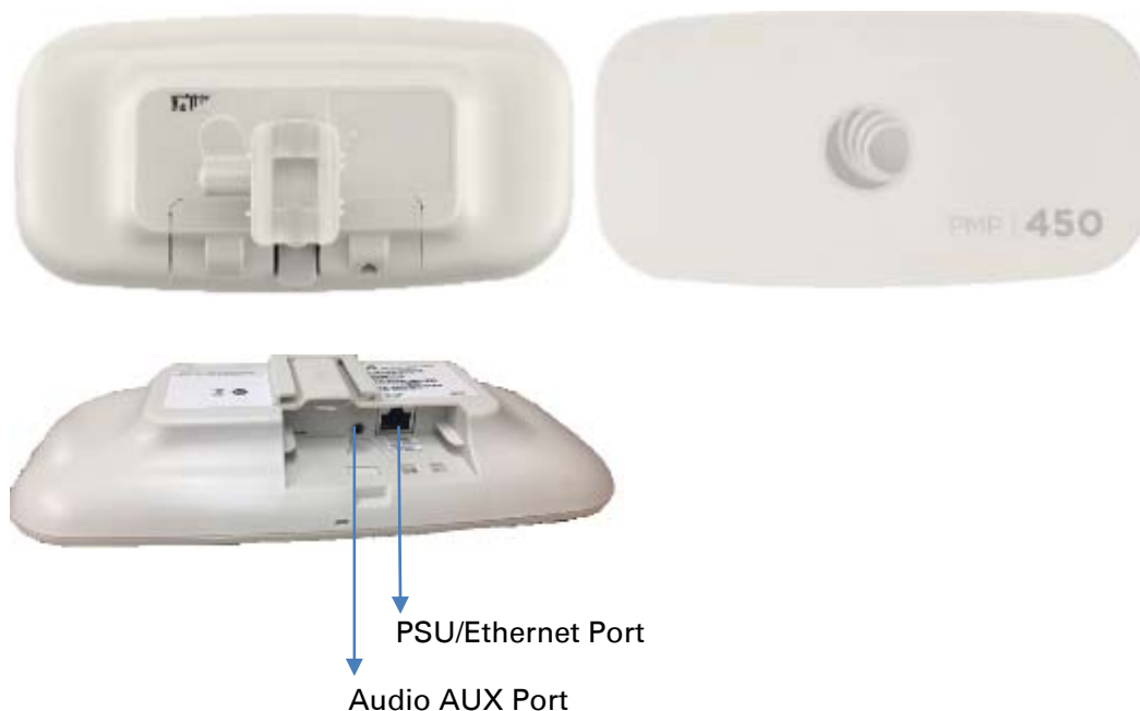
Figure 5 PMP 450b Series - SM interfaces
