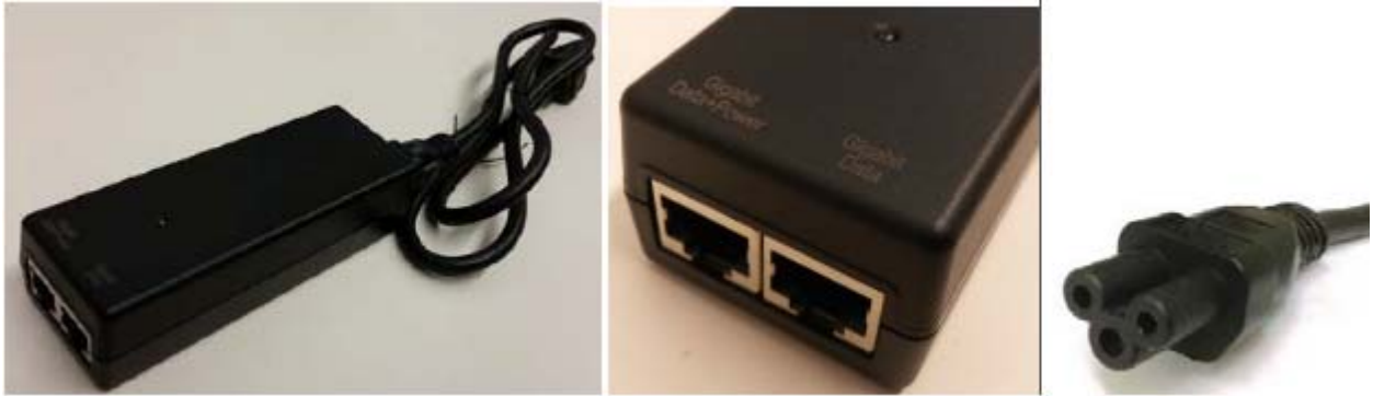
Figure 19 Gigabit Enet Capable power supply
