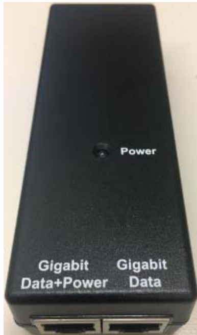
Figure 18 -20 to 32 VDC Power Injector interfaces
