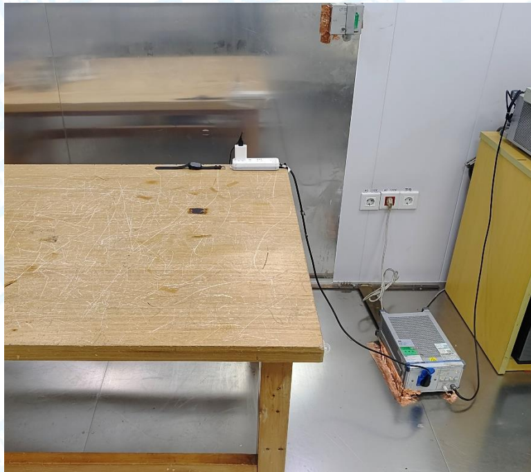
Photo of Setup for Conducted Emission
