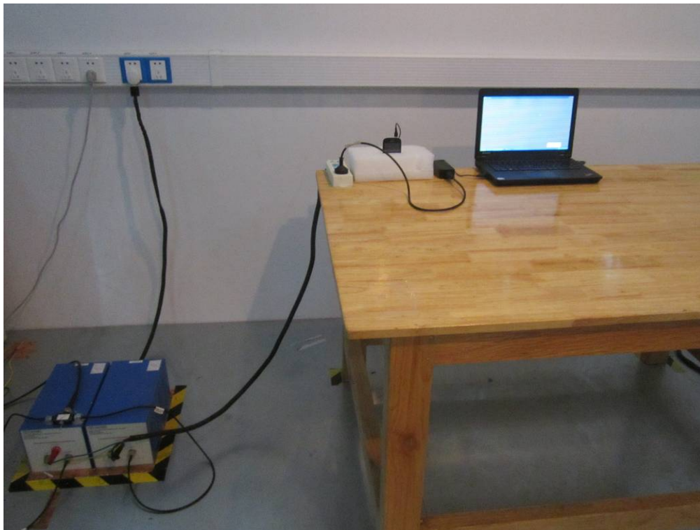
Conducted Emissions Test Setup Front View
