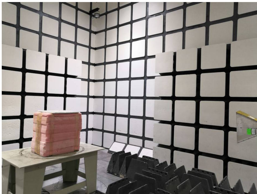
Radiated Emissions View (Above 1 GHz)
