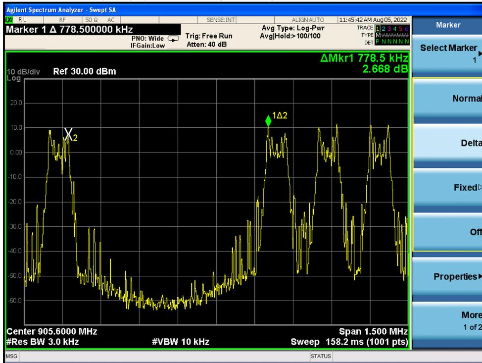
(1Mbps) Channel Separation plot on channel 52-53
