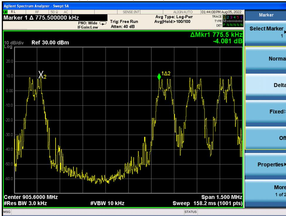
(1Mbps) Channel Separation plot on channel 52-53
