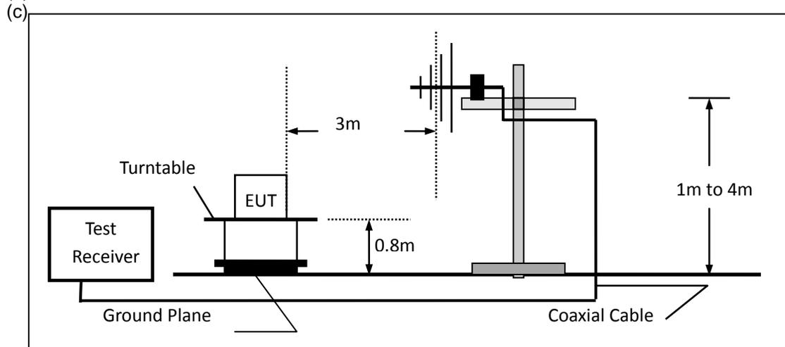
(c) For radiated emissions above 1000MHz
