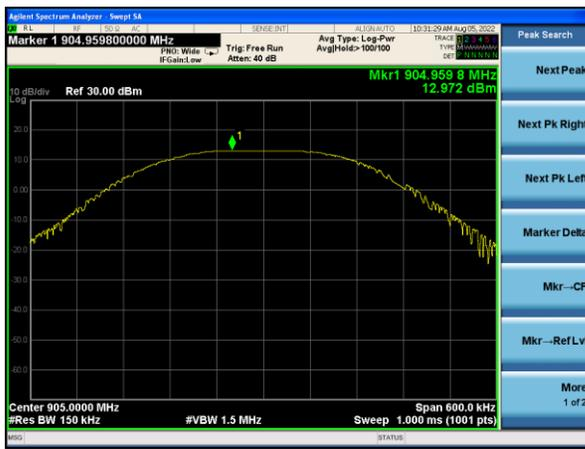
Peak output Power plot on channel 52 (1Mbps)
