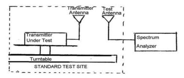
b) Raise and lower the test antenna from 1m to 4m and rotate turntable from 0° to 360°. Record the highest received signal showed in spectrum analyzer as Rt . Calculate electric field strength in receive antenna as Et.
