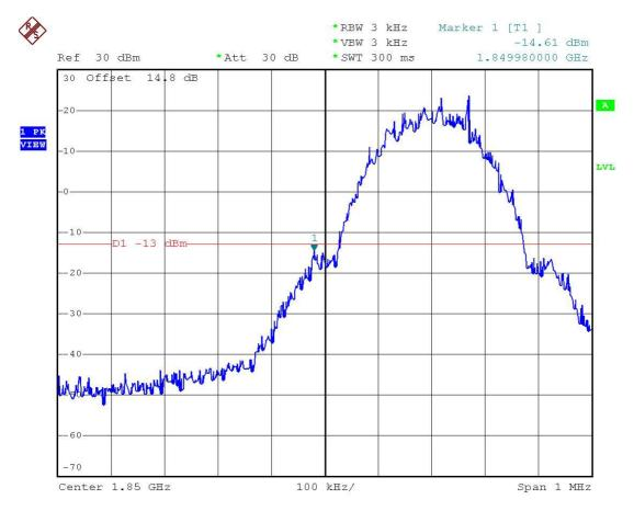
**Name of Test**: Emission Masks (Occupied Bandwidth) State 2:High Power
