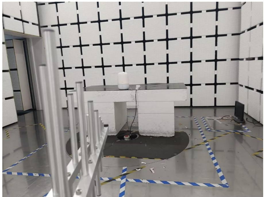
Radiation Emission Test Setup (30MHz to 1GHz)
