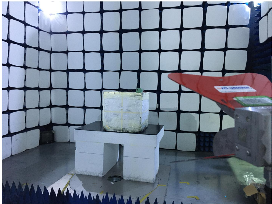
Radiation Emission Test Setup (1GHz to 18GHz)
