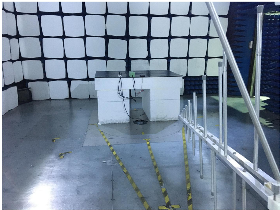
Radiation Emission Test Setup (30MHz to 1GHz)
