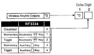
The outputs may be assigned to follow the Keyfobs in one or all partitions in the Output Partition Assignment Addresses 0149-0150.
