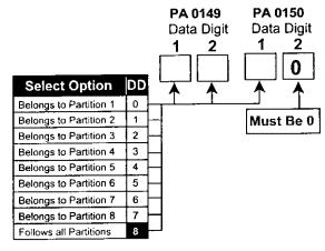
Programming the Output Functions to follow the wireless keypad accessory 🕷 key.
