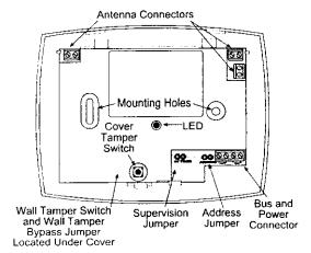
Install anchors where studs are not present and secure the receiver base to the wall with screws at the mounting hole locations. Insert an antenna into the outside terminal on two of the antenna terminal blocks.
