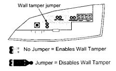
For UL Certificated Installations, tamper switches must be enabled.
