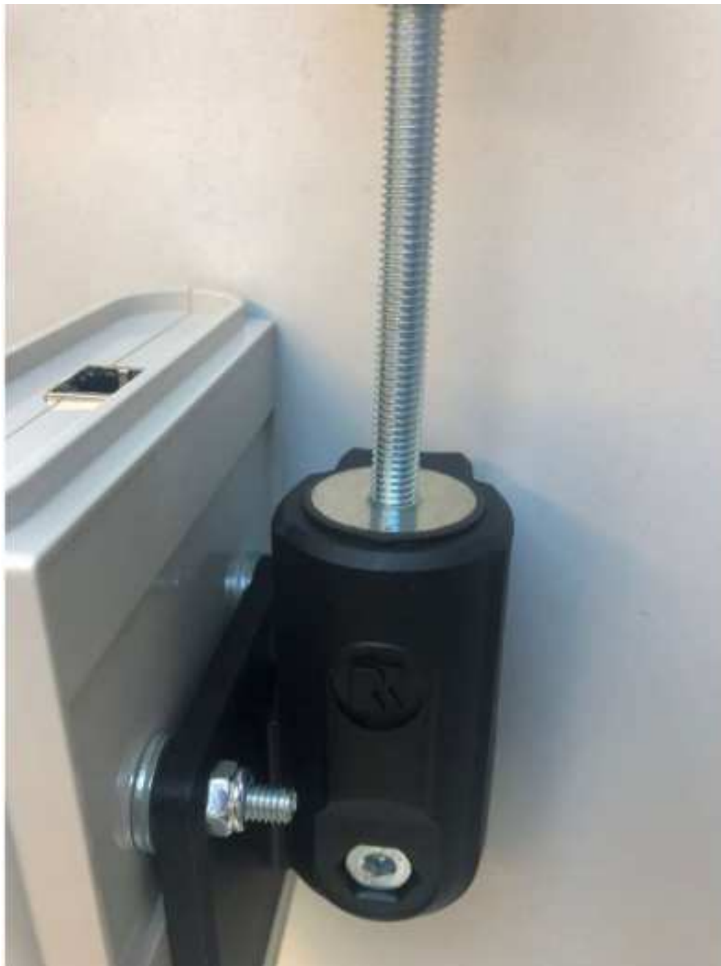
Figure 1: Articulated arm with threaded rod screwed in
