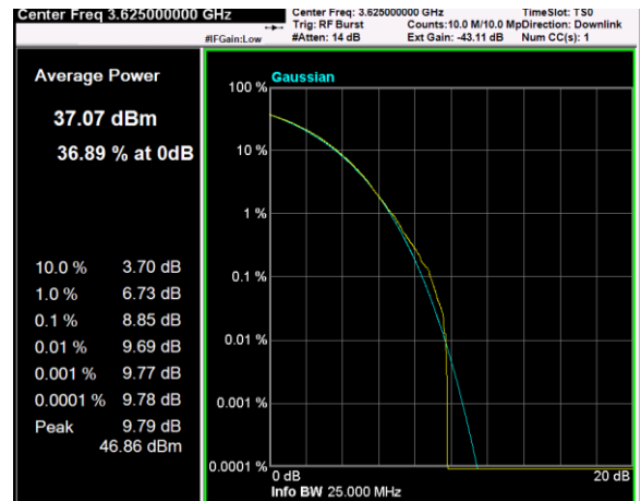
Channel: MIDDLE, Modulation: QPSK, BW=20MHz, CCDF
