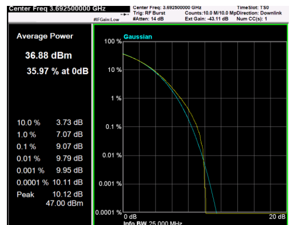
Channel: TOP, Modulation: 256QAM, BW=15MHz, CCDF
