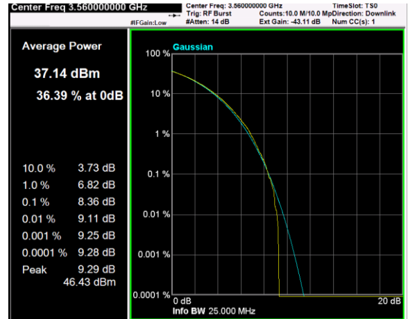
Channel: BOTTOM, Modulation: QPSK, BW=20MHz, CCDF
