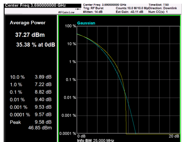
Channel: TOP, Modulation: 256QAM, BW=20MHz, CCDF
