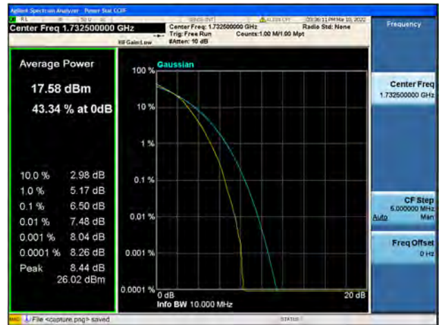
Band4 / 10MHz / High CH / QPSK
