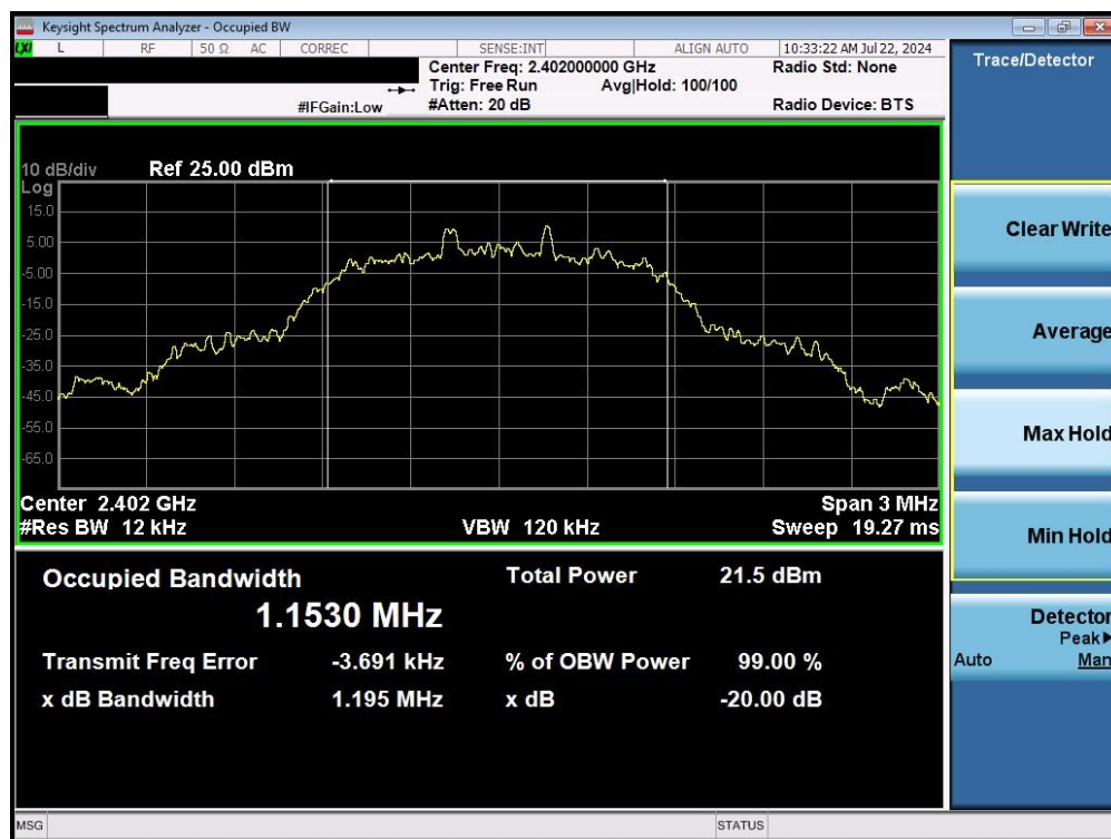
Plot 7-4. 20dB BW and 99% OBW Plot (Bluetooth, 8DPSK, Ch. 0)
