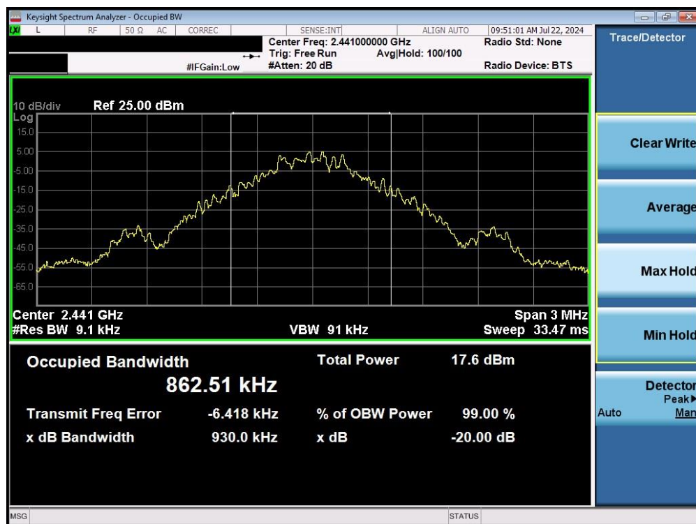
Plot 7-2. 20dB BW and 99% OBW Plot (Bluetooth, GFSK, Ch. 39)
