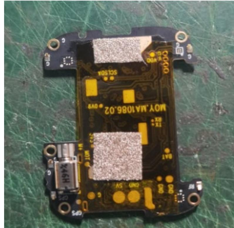
2, the motherboard copper leakage area paste sponge and battery grounding
