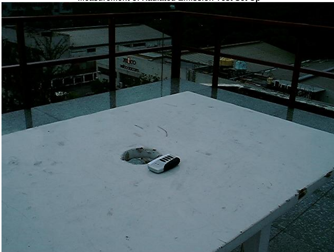
Measurement of Radiated Emission Test Set Up
