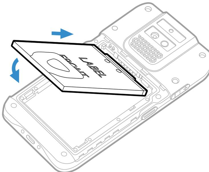
2. Insert the battery cover into the computer.
