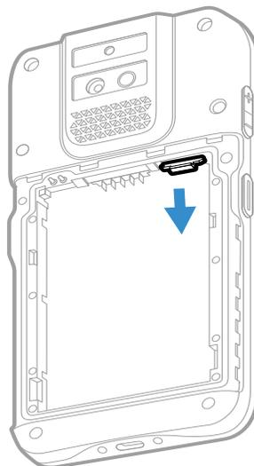
5. Place the nanoSIM card into the card holder tray with contacts facing down.
