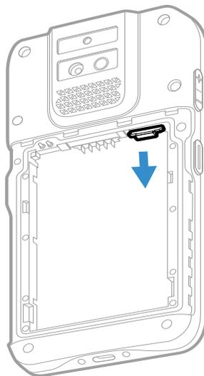
6. Insert the microSD card into the card holder tray with the contacts facing down.
