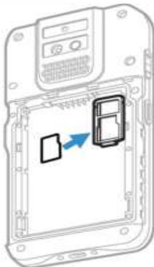
7. Slide the card holder tray back into the slot.
