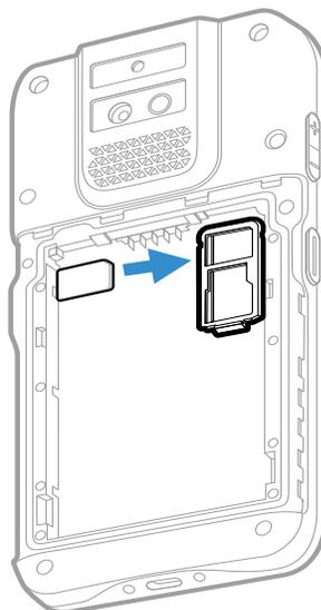
6. Slide the card holder tray back into the card holder slot.
