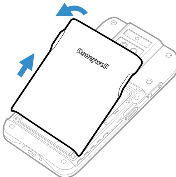
4. Pull up the tab on the back of the battery to lift and remove it from the computer.
