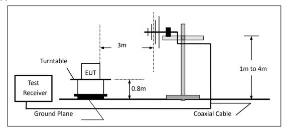
(c) For radiated emissions above 1000MHz
