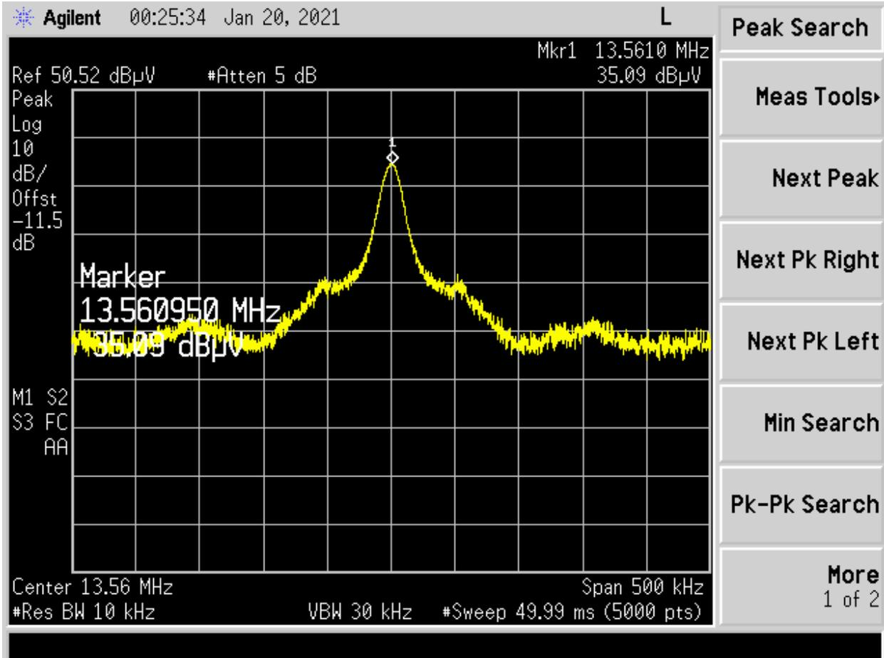
Graph 4: Frequency Tolerance Cold (-20° C)
