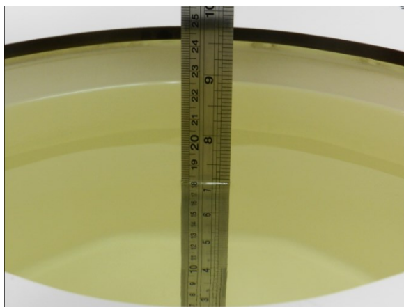
Fig 11.1 Photo of Liquid Height for Body SAR
