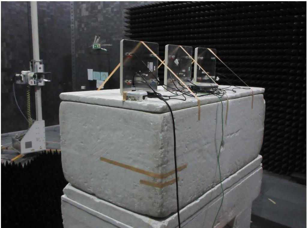
For radiated emissions 30MHz~1GHz
