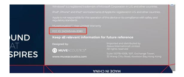
Because the product is a wireless headset, the product area is too small to print FCC ID, so according to the regulatory requirements, the FCC ID number is printed on the manual and color box, as shown in the screenshot above.
