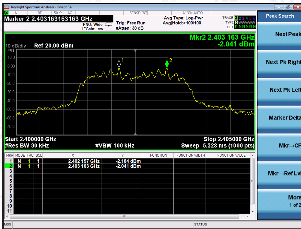
TEST PLOT FOR FREQUENCY SEPARATION
