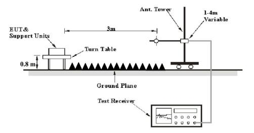
The radiated emission tests were performed in the 3 meters, using the setup accordance with the ANSI C63.17-2013. The specification used was the FCC 15.209 and FCC 15.319 (g) limits.
