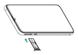
When inserting your card tray, make sure that the card tray is level and that the card is aligned correctly.
