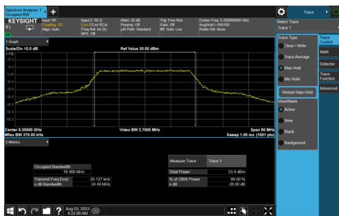
Plot 7-2. 26dB BW & 99% OBW (20MHz BW 802.11n – Ch. 40, MCS0)
