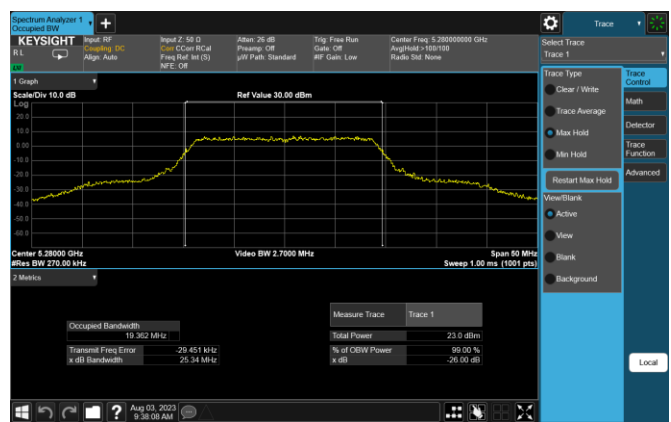
Plot 7-5. 26dB BW & 99% OBW (20MHz BW 802.11n – Ch. 56, MCS0)
