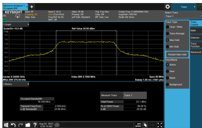
Plot 7-3. 26dB BW & 99% OBW (20MHz BW 802.11n – Ch. 48, MCS0)
