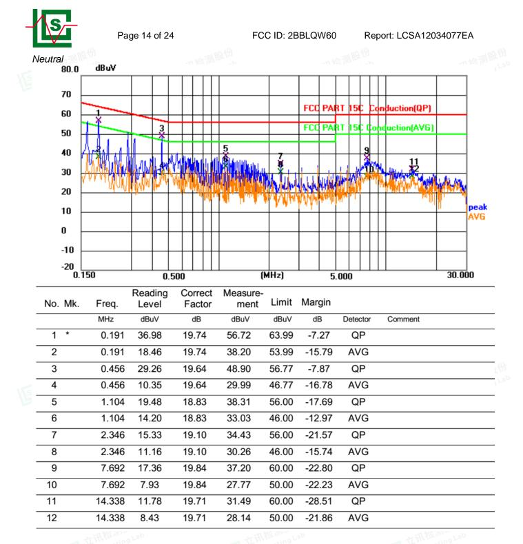
\*\*\*Note: Pre-scan all modes and recorded the worst case results in this report. Margin=Reading level + Correct - Limit; Correct Factor= Lisn Factor+Cable Factor
