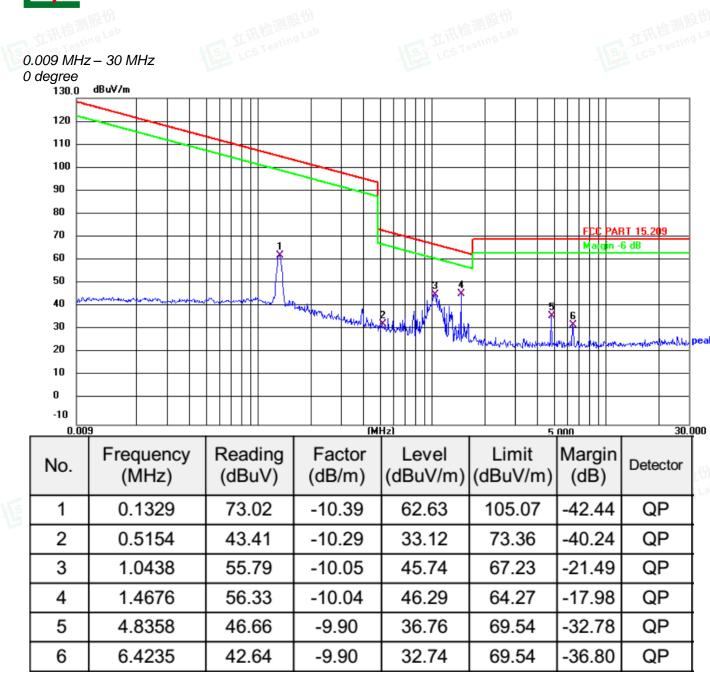
Remark: 1). Measured at antenna position 0 degree and 90 degree, recorded worst case at 0 degree. 2). Margin=Reading level + Factor- Limit
