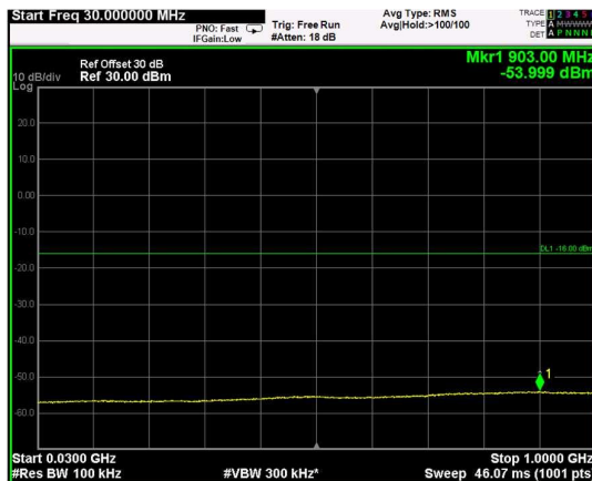
Channel: TOP, Modulation: QPSK, BW=15MHz, Range: Lower
