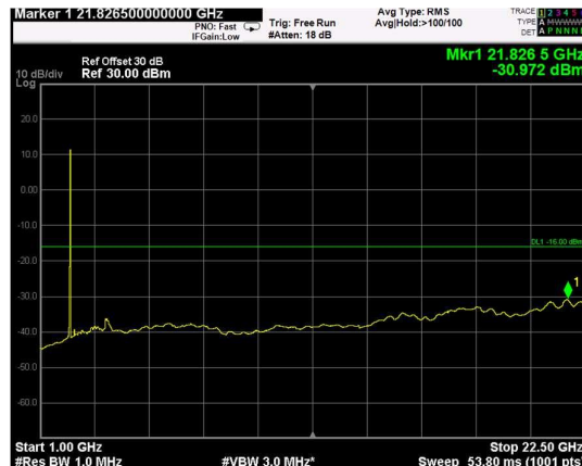
Channel: MIDDLE, Modulation: 256QAM, BW=10MHz, Range: Upper
