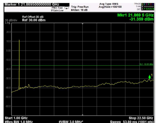
Channel: TOP, Modulation: 64QAM, BW=10MHz, Range: Upper
