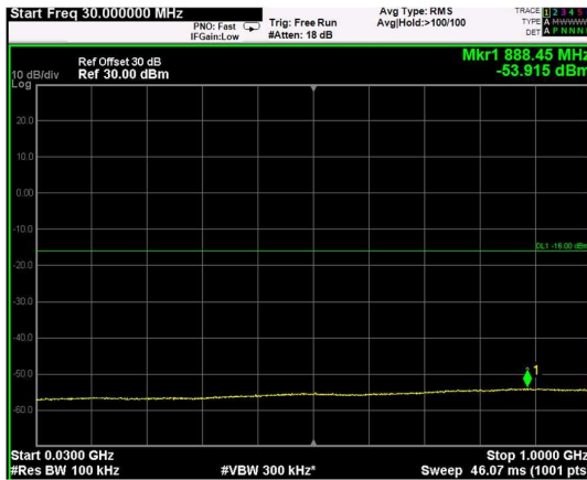
Channel: BOTTOM, Modulation: QPSK, BW=10MHz, Range: Lower
