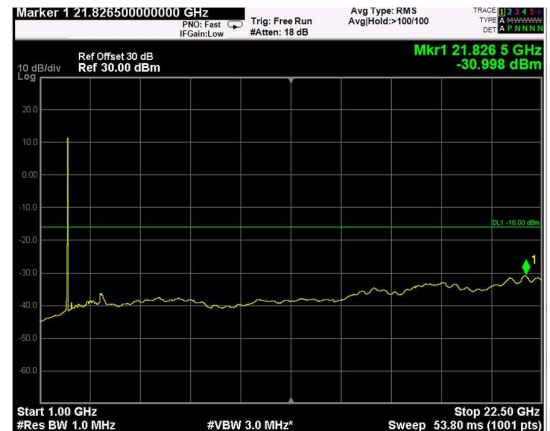
Channel: MIDDLE, Modulation: 64QAM, BW=10MHz, Range: Upper
