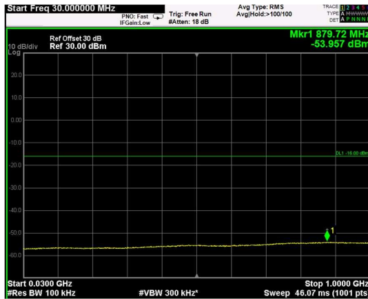
Channel: MIDDLE, Modulation: QPSK, BW=15MHz, Range: Lower
