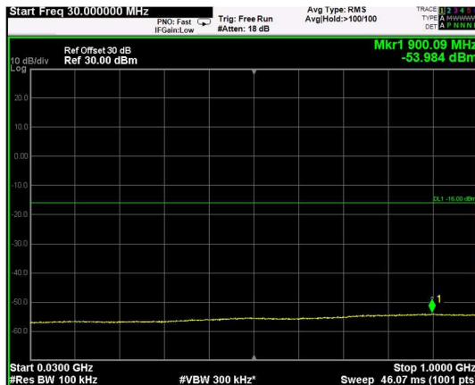
Channel: MIDDLE, Modulation: 256QAM, BW=15MHz, Range: Lower
