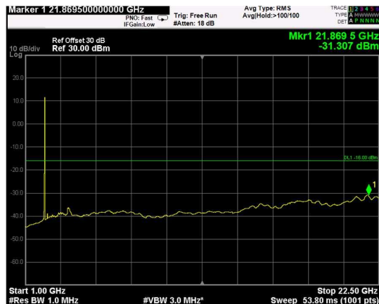
Channel: TOP, Modulation: 16QAM, BW=15MHz, Range: Upper
