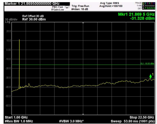
Channel: BOTTOM, Modulation: 64QAM, BW=5MHz, Range: Upper
