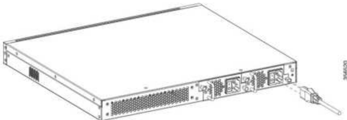
Figure 17: Connecting an AC Power Cable to CGP-OLT-16T
