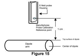
Separation Distance from Dipole to Field Probe
