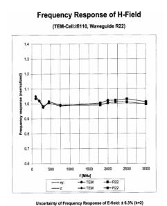
Figure 9 H-Field Probe Frequency Response
