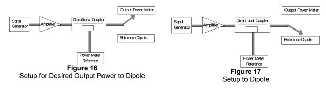
Using this setup configuration, the signal generator was adjusted for the desired output power (100mW) at a specified frequency. The reference power from the coupled port of the directional coupler is recorded. Next, the output cable is connected to the reference dipole, as shown in Figure 17.
