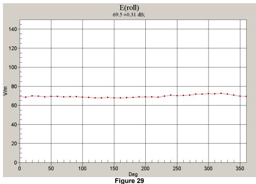
Worst-Case Probe Rotation about Azimuth axis
