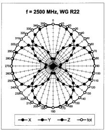
Receiving Pattern ( $\phi$ ),  $\vartheta = 90^{\circ}$
