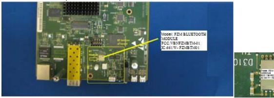
Identification label placed on FZM unit level externally as shown below.
