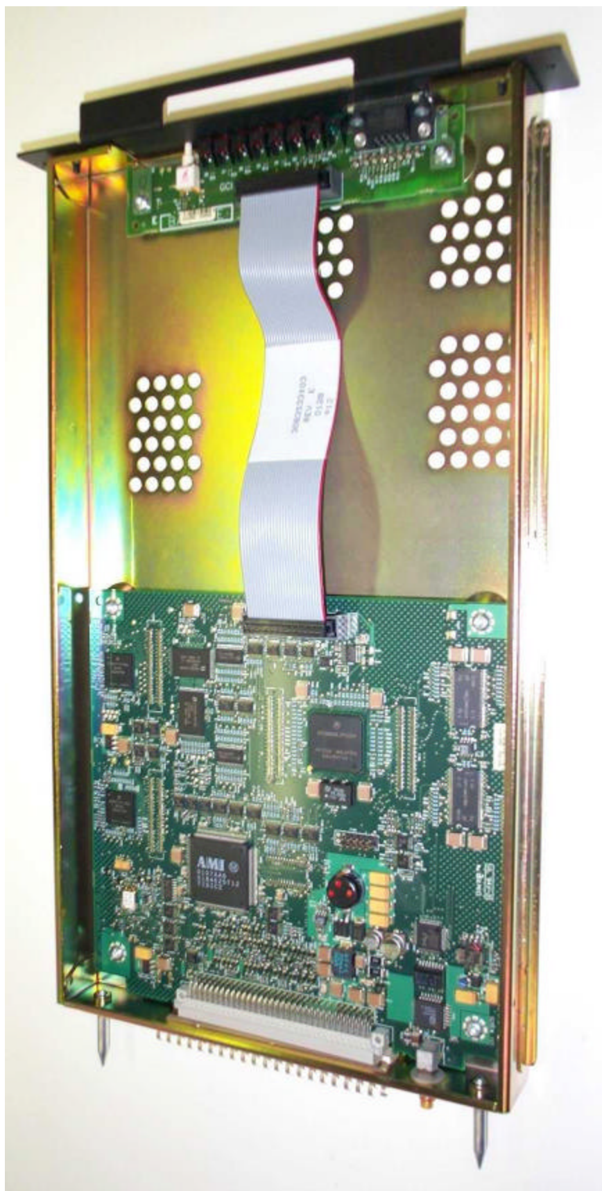
Enhanced Base Radio Control Module, Top Side
