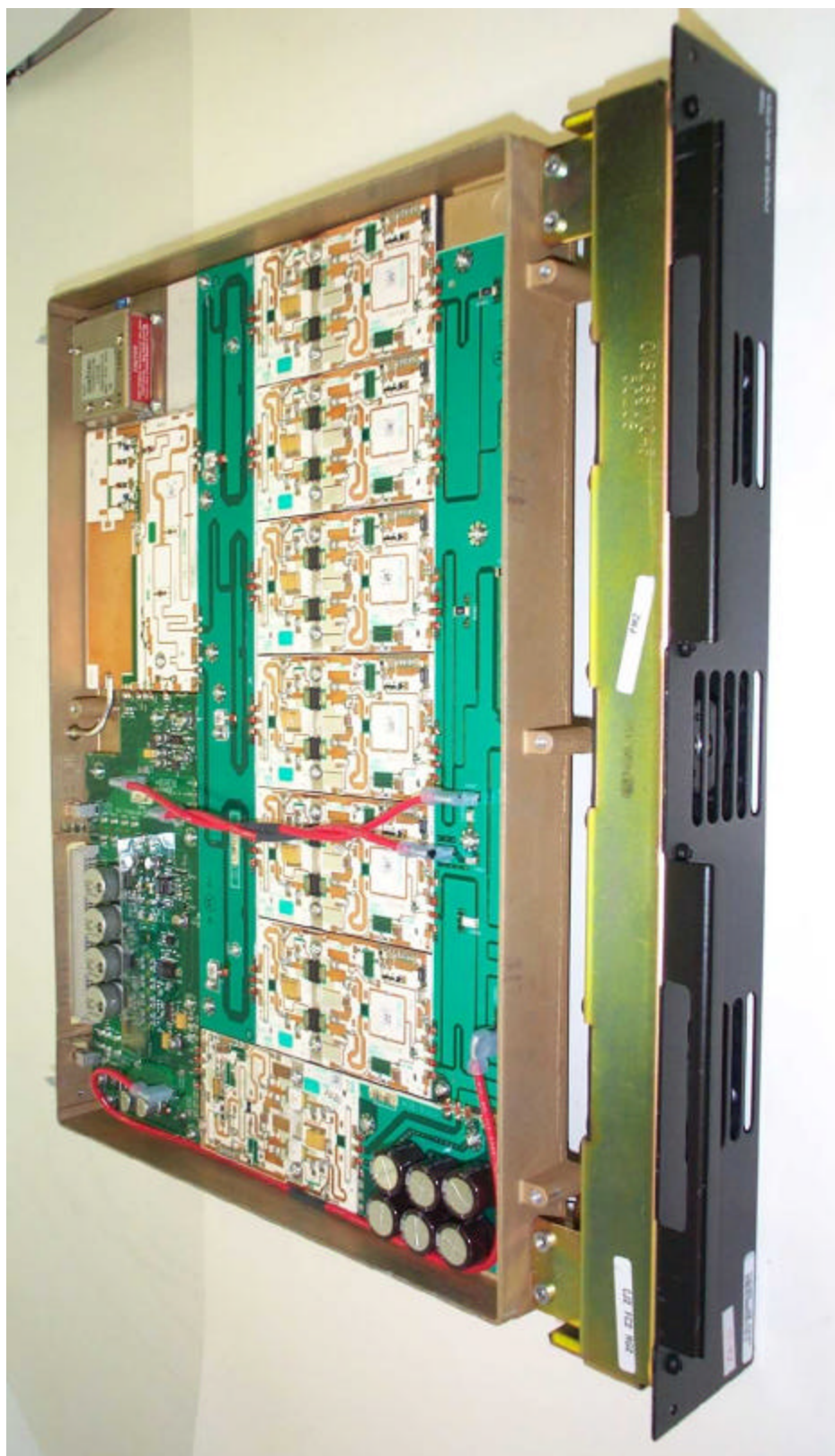
Power Amplifier Module, Top View, Shields Removed
