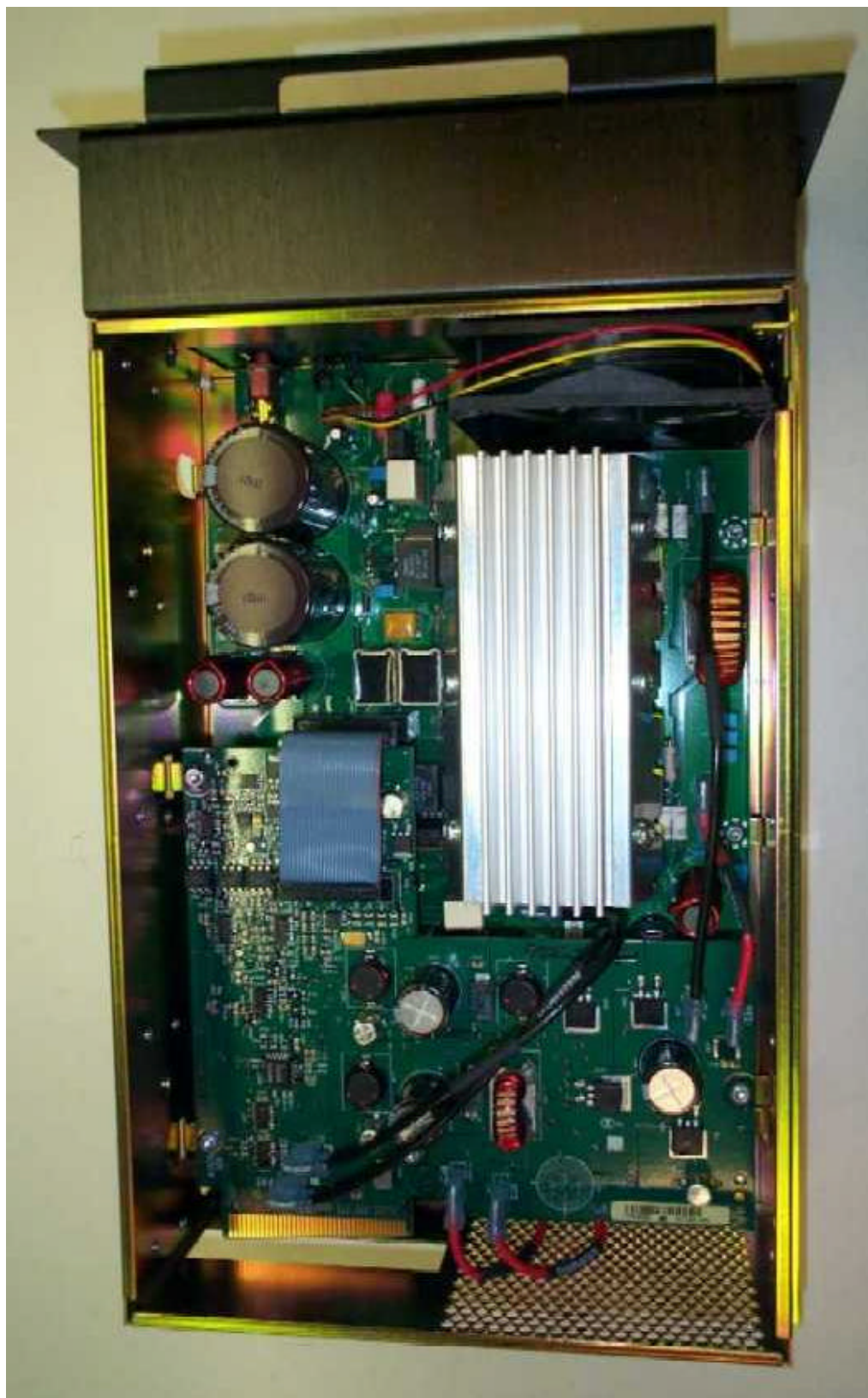
Power Supply Module, Cover Removed
