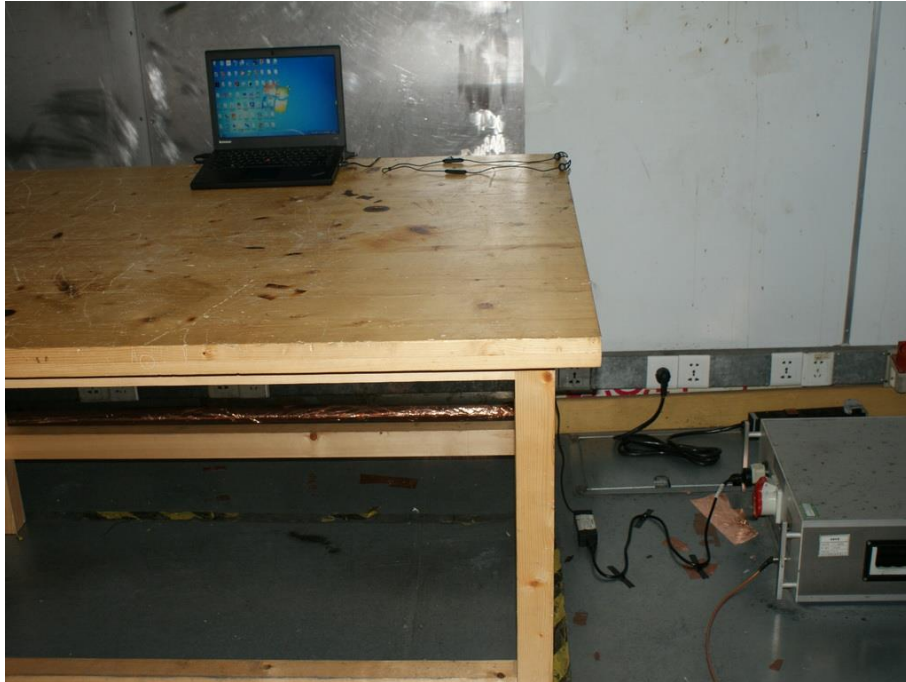
Photograph 1: Set-up for Conducted Emission on AC Mains
