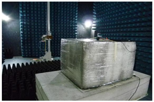
Radiated Emission Set up Photos (Front View)
