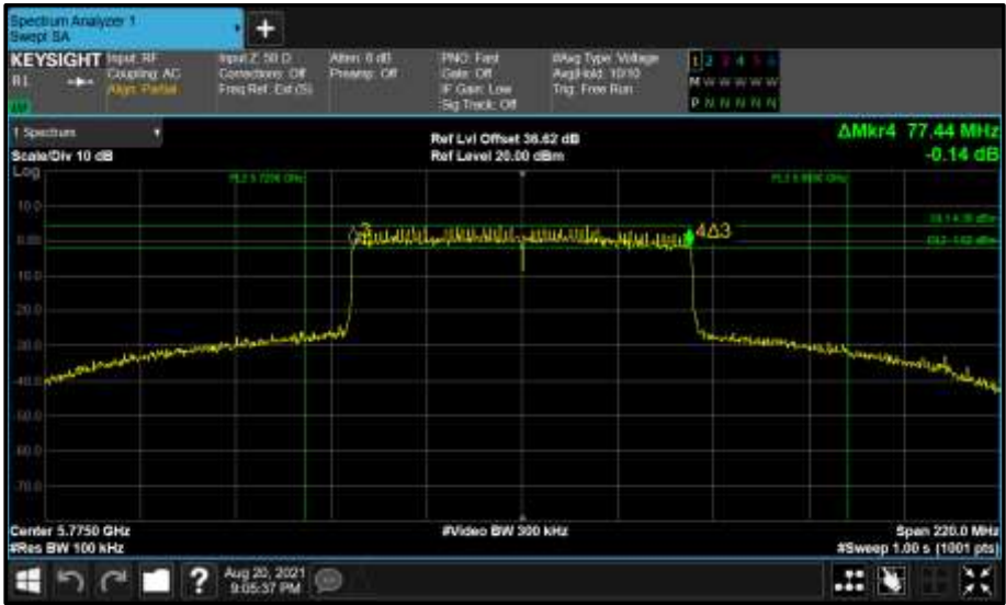
Figure 890 - Core 1 (B) 5775 MHz (CH155) 6 dB Bandwidth
