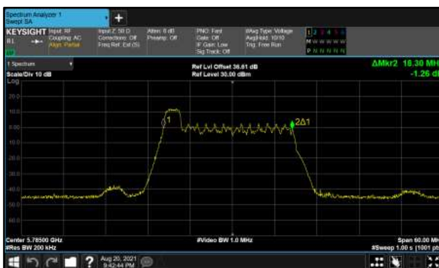
Figure 763 - Core 1 (B) 5785 MHz (CH157) 99% Bandwidth
