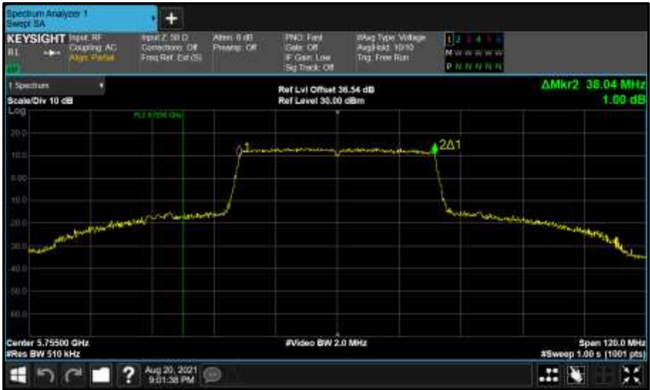
Figure 859 - Core 0 (A) 5755 MHz (CH151) 99% Bandwidth
