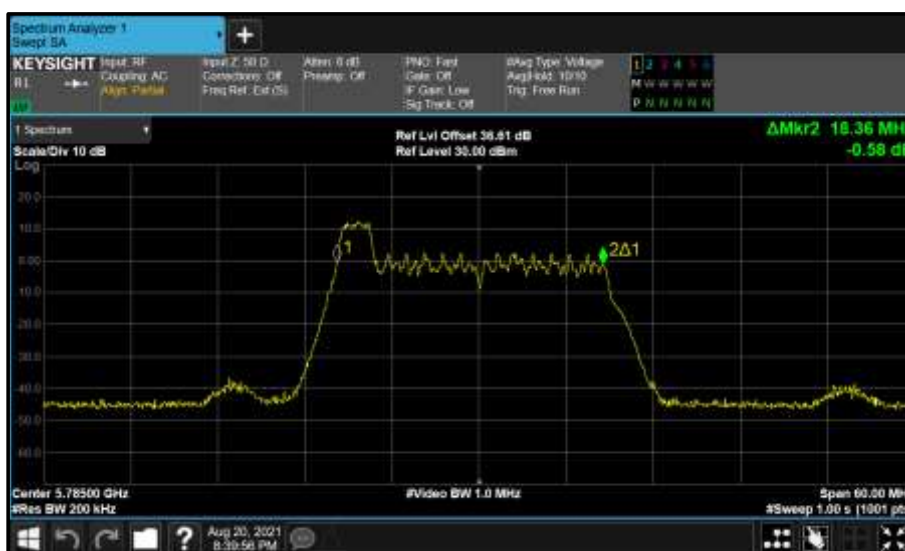
Figure 741 - Core 1 (B) 5785 MHz (CH157) 99% Bandwidth
