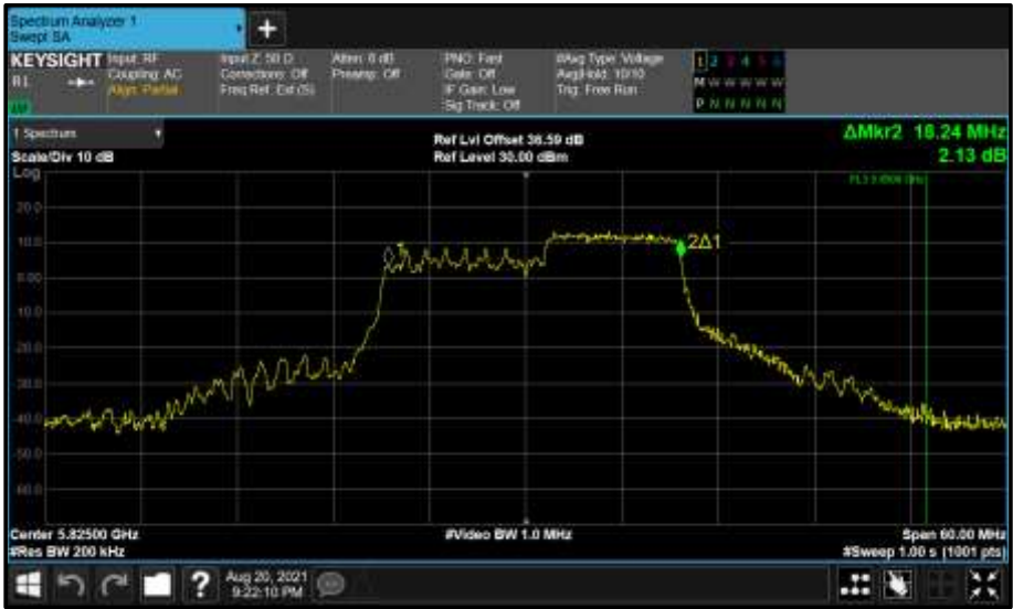
Figure 831 - Core 1 (B) 5825 MHz (CH165) 99% Bandwidth
