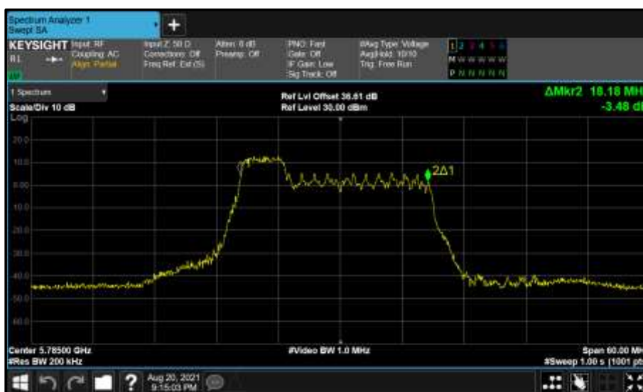
Figure 787 - Core 1 (B) 5785 MHz (CH157) 99% Bandwidth
