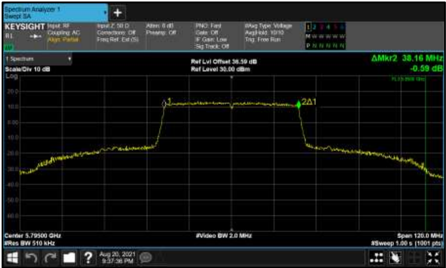
Figure 875 - Core 0 (A) 5795 MHz (CH159) 99% Bandwidth
