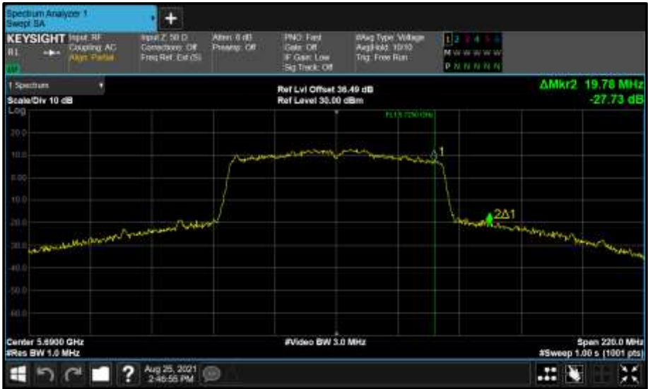
Figure 693 - Core 1 (B) 5690 MHz (CH138) 99% Bandwidth
