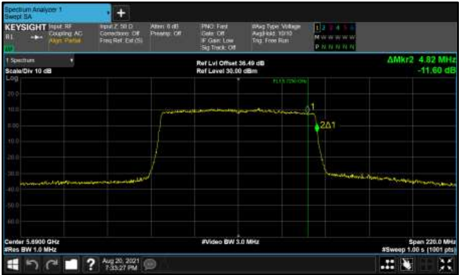
Figure 885 - Core 1 (B) 5690 MHz (CH138) 99% Bandwidth
