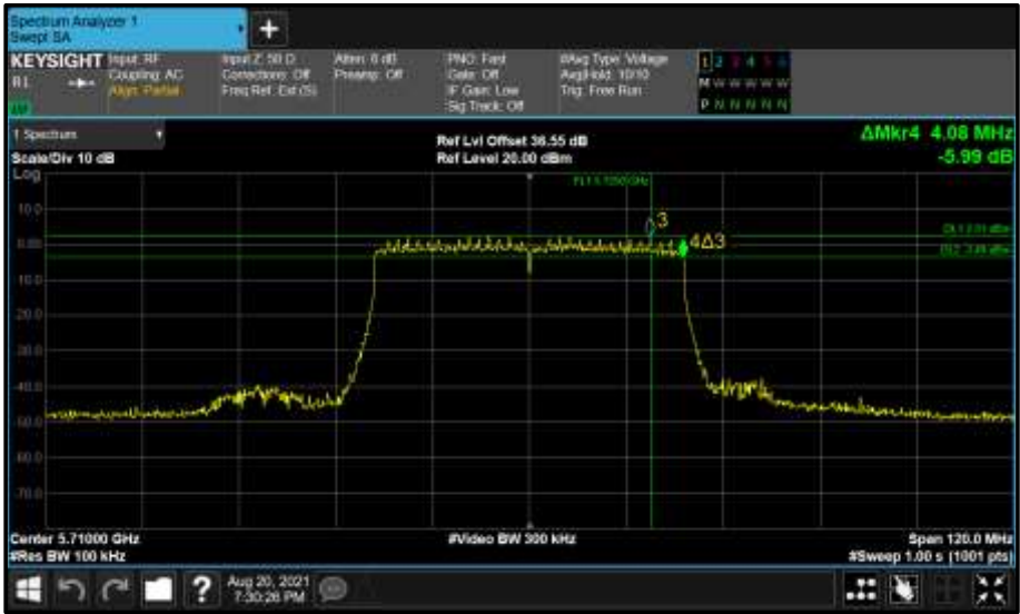
Figure 858 - Core 1 (B) 5710 MHz (CH142) 6 dB Bandwidth
