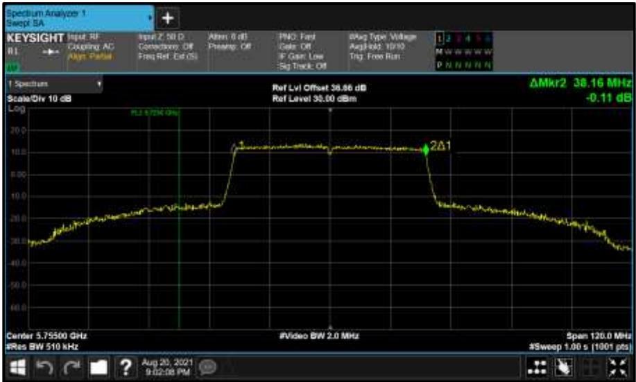
Figure 861 - Core 1 (B) 5755 MHz (CH151) 99% Bandwidth
