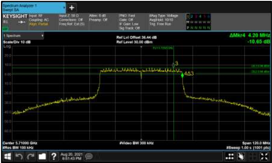
Figure 850 - Core 0 (A) 5710 MHz (CH142) 6 dB Bandwidth
