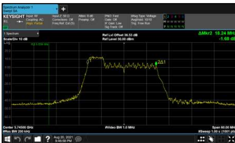
Figure 797 - Core 0 (A) 5745 MHz (CH149) 99% Bandwidth
