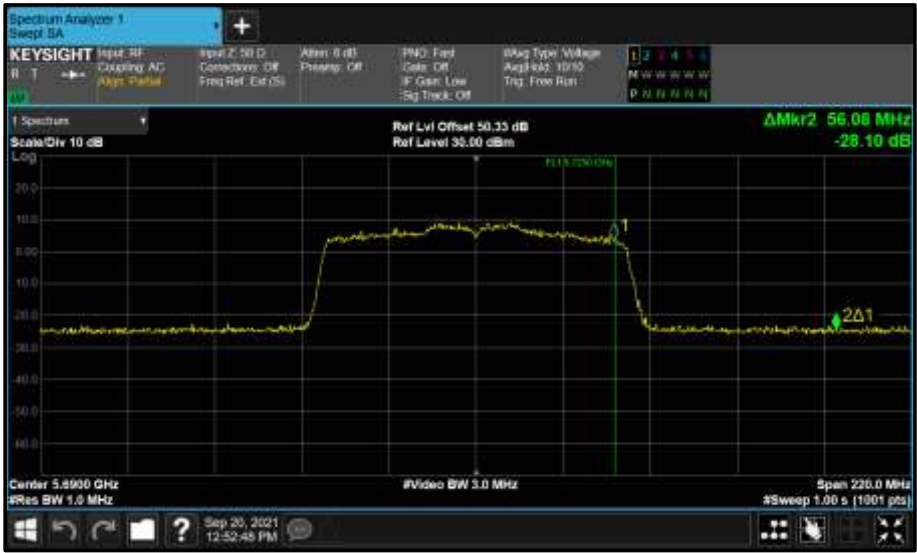
Figure 927 - Core 0 (A) 5690 MHz (CH138) 99% Bandwidth
