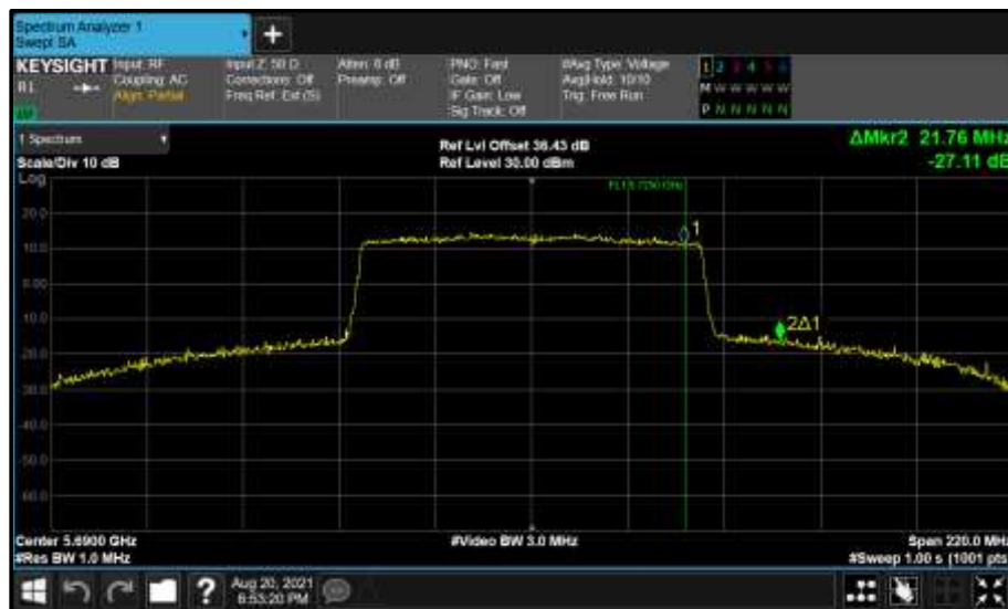
Figure 879 - Core 0 (A) 5690 MHz (CH138) 99% Bandwidth
