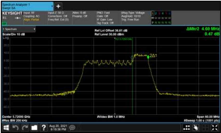
Figure 795 - Core 1 (B) 5720 MHz (CH144) 99% Bandwidth
