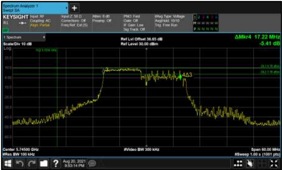
Figure 840 - Core 1 (B) 5745 MHz (CH149) 6 dB Bandwidth
