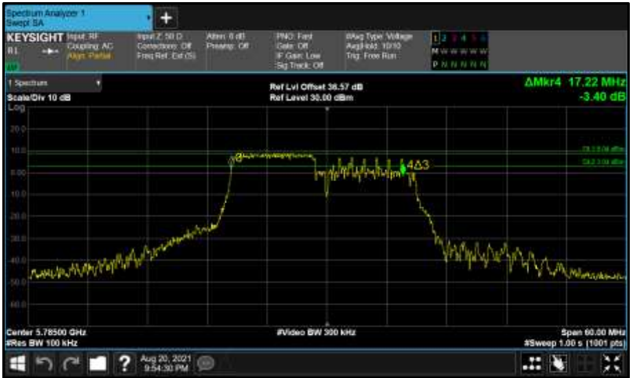
Figure 842 - Core 0 (A) 5785 MHz (CH157) 6 dB Bandwidth
