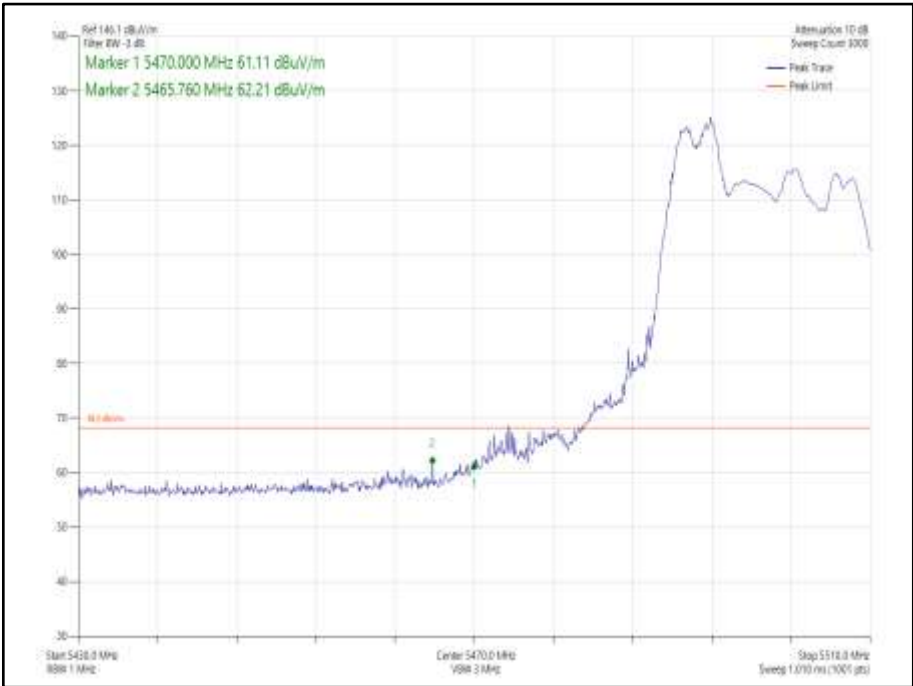
Figure 954 - 802.11ax HE20 CDD, Cores 0-1 52-37 - 5500 MHz Band Edge Frequency 5470 MHz
