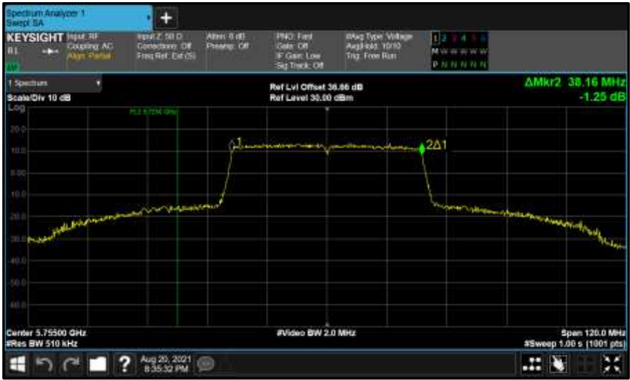
Figure 851 - Core 1 (B) 5755 MHz (CH151) 99% Bandwidth
