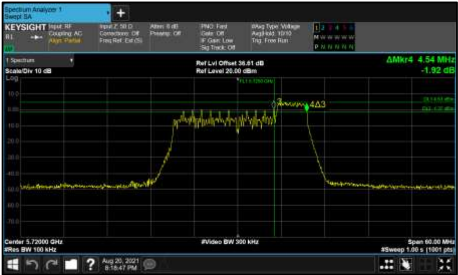
Figure 796 - Core 1 (B) 5720 MHz (CH144) 6 dB Bandwidth
