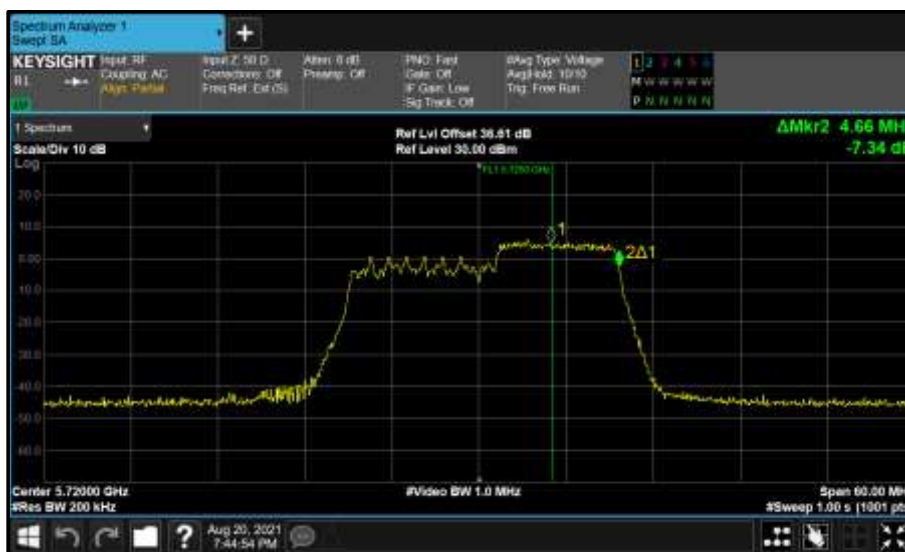
Figure 819 - Core 1 (B) 5720 MHz (CH144) 99% Bandwidth
