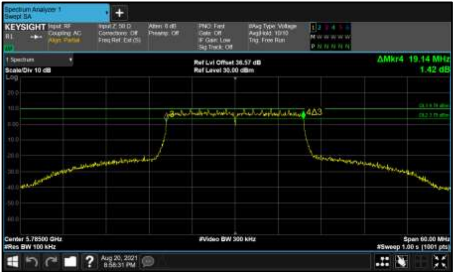
Figure 716 - Core 0 (A) 5785 MHz (CH157) 6 dB Bandwidth
