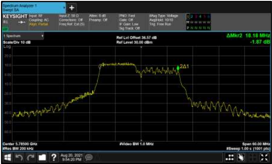
Figure 841 - Core 0 (A) 5785 MHz (CH157) 99% Bandwidth
