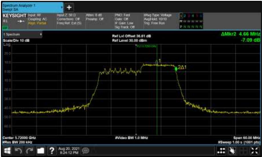
Figure 835 - Core 1 (B) 5720 MHz (CH144) 99% Bandwidth
