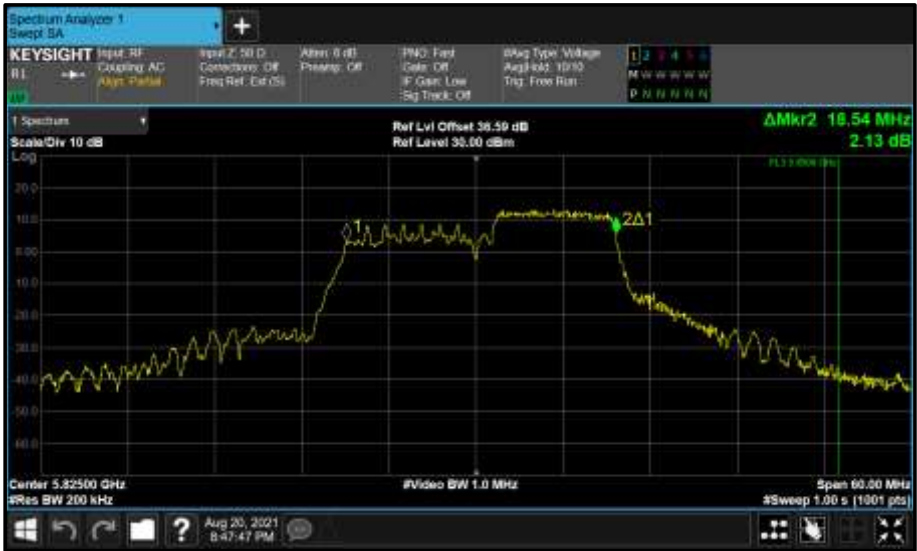
Figure 815 - Core 1 (B) 5825 MHz (CH165) 99% Bandwidth
