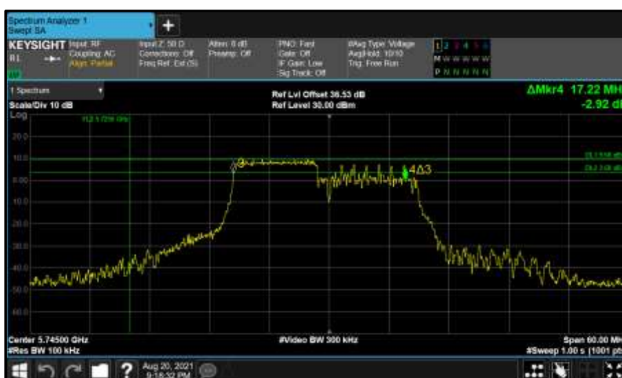
Figure 822 - Core 0 (A) 5745 MHz (CH149) 6 dB Bandwidth
