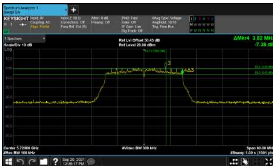
Figure 900 - Core 0 (A) 5720 MHz (CH144) 6 dB Bandwidth
