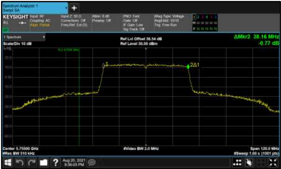
Figure 871 - Core 0 (A) 5755 MHz (CH151) 99% Bandwidth
