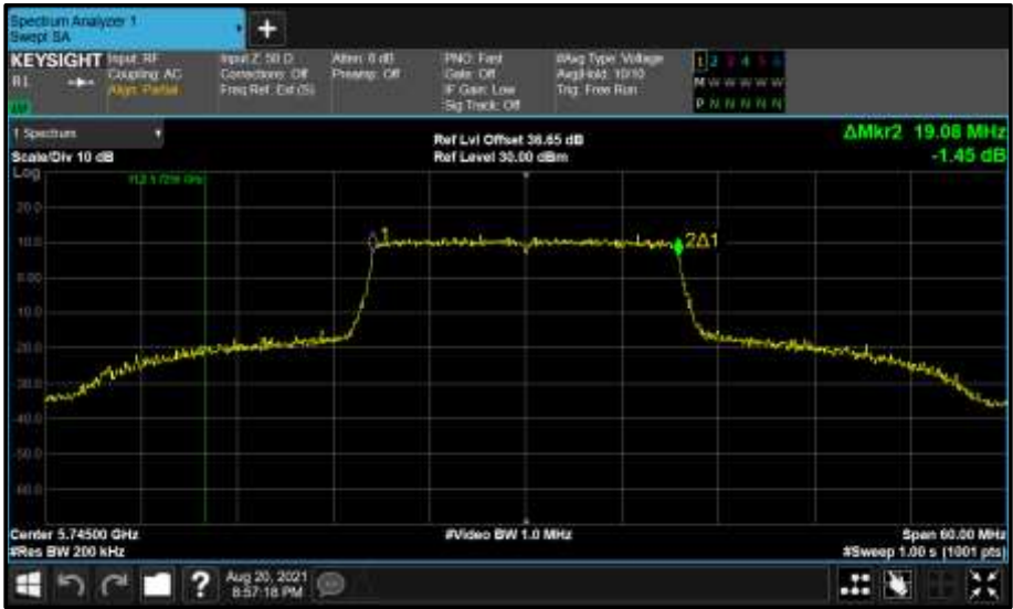
Figure 713 - Core 1 (B) 5745 MHz (CH149) 99% Bandwidth
