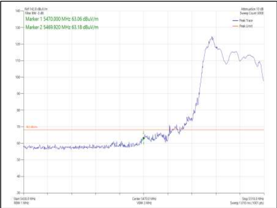
Figure 956 - 802.11ax HE20 SDM, Cores 0-1 52-37 - 5500 MHz Band Edge Frequency 5470 MHz
