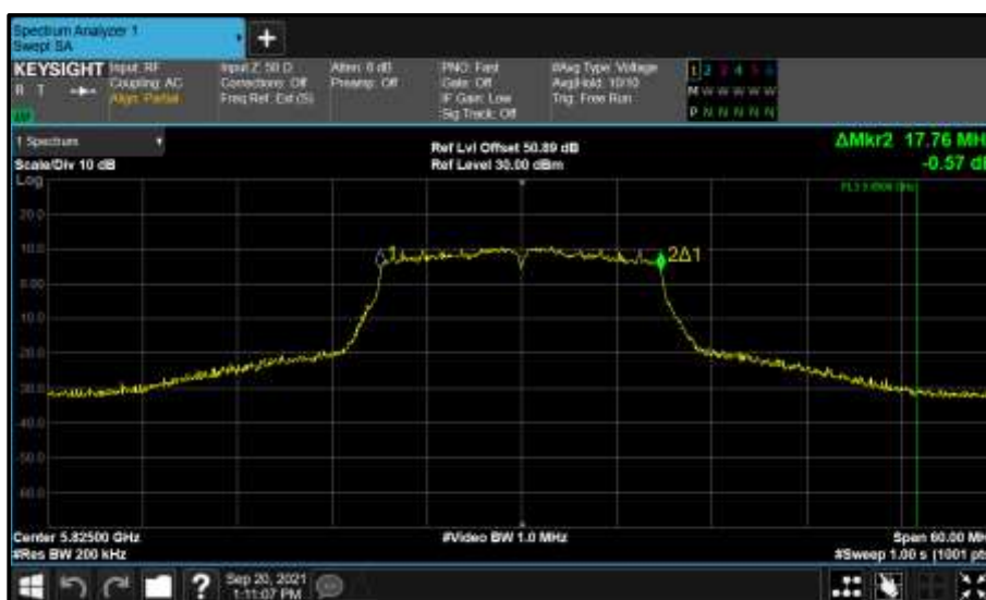
Figure 913 - Core 1 (B) 5825 MHz (CH165) 99% Bandwidth
