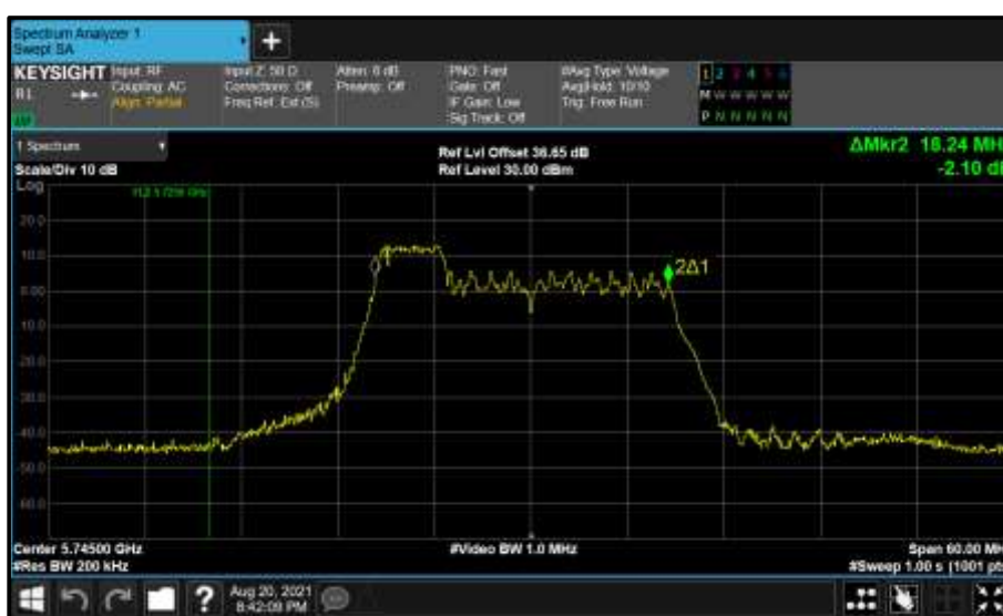
Figure 771 - Core 1 (B) 5745 MHz (CH149) 99% Bandwidth
