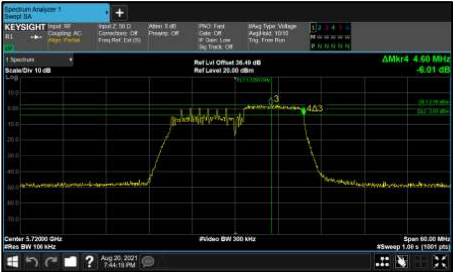
Figure 818 - Core 0 (A) 5720 MHz (CH144) 6 dB Bandwidth
