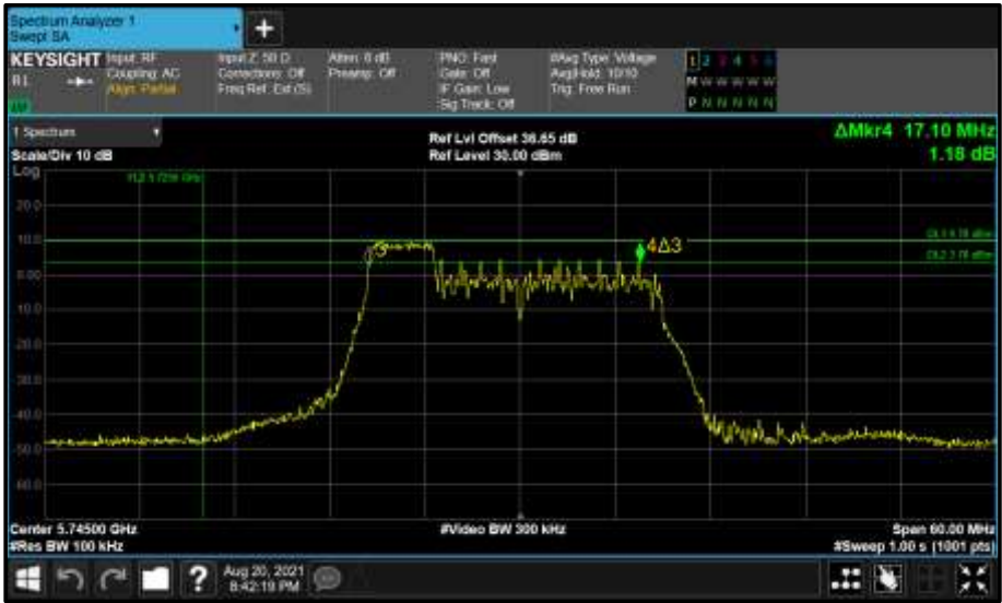
Figure 772 - Core 1 (B) 5745 MHz (CH149) 6 dB Bandwidth
