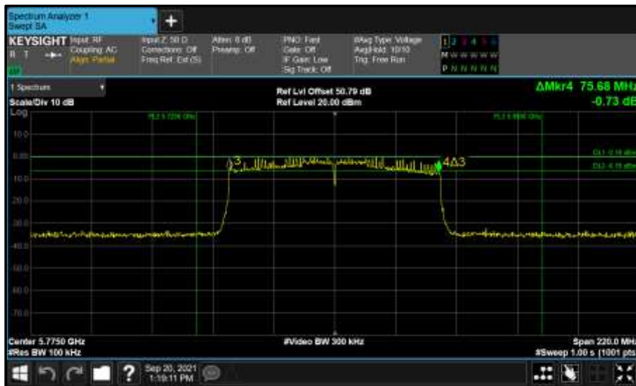
Figure 934 - Core 1 (B) 5775 MHz (CH155) 6 dB Bandwidth
