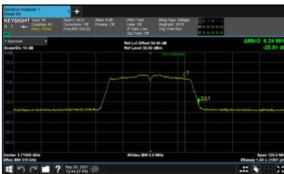
Figure 915 - Core 0 (A) 5710 MHz (CH142) 99% Bandwidth
