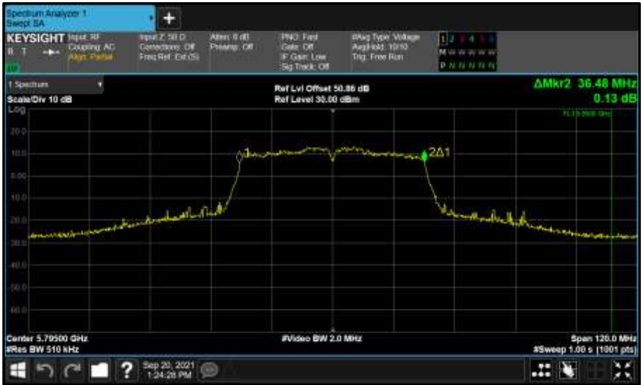
Figure 925 - Core 1 (B) 5795 MHz (CH159) 99% Bandwidth
