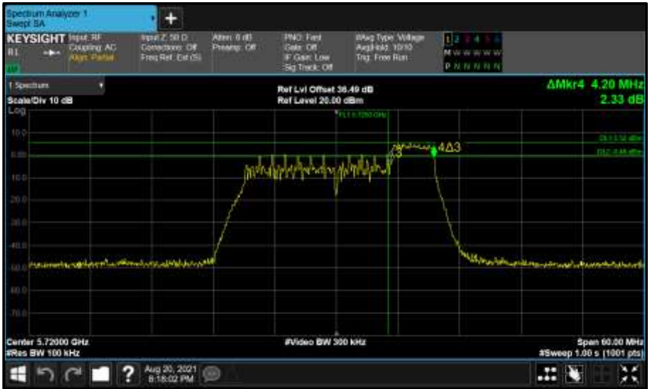
Figure 794 - Core 0 (A) 5720 MHz (CH144) 6 dB Bandwidth
