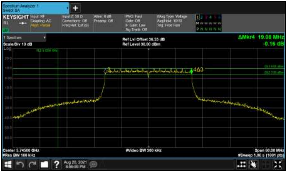
Figure 712 - Core 0 (A) 5745 MHz (CH149) 6 dB Bandwidth
