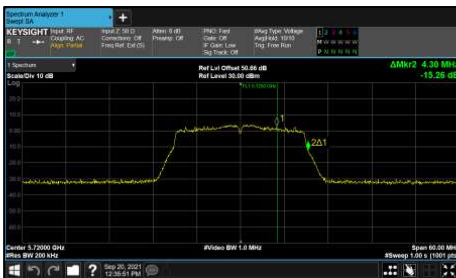
Figure 901 - Core 1 (B) 5720 MHz (CH144) 99% Bandwidth
