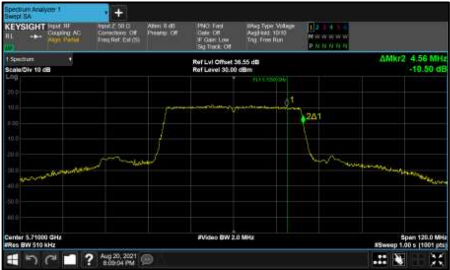
Figure 869 - Core 1 (B) 5710 MHz (CH142) 99% Bandwidth
