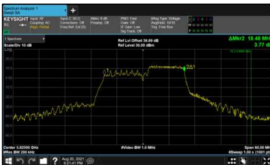
Figure 829 - Core 0 (A) 5825 MHz (CH165) 99% Bandwidth
