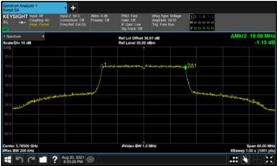
Figure 703 - Core 1 (B) 5785 MHz (CH157) 99% Bandwidth
