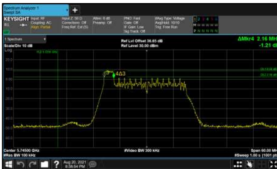
Figure 740 - Core 1 (B) 5745 MHz (CH149) 6 dB Bandwidth
