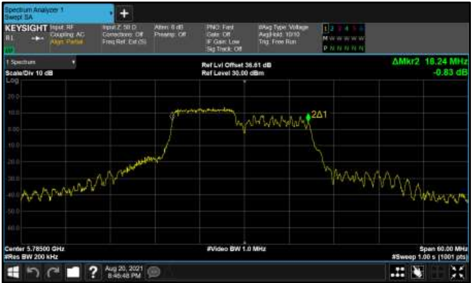
Figure 813 - Core 1 (B) 5785 MHz (CH157) 99% Bandwidth
