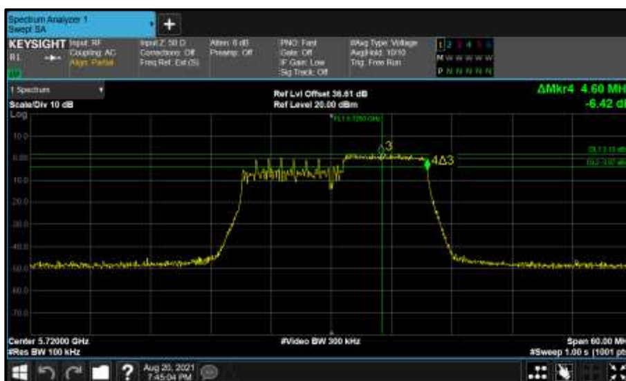
Figure 820 - Core 1 (B) 5720 MHz (CH144) 6 dB Bandwidth
