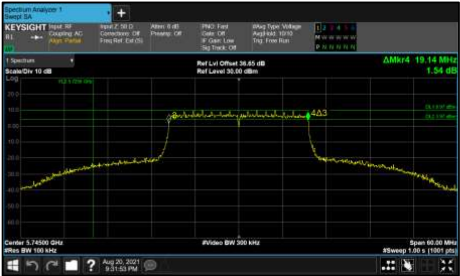
Figure 730 - Core 1 (B) 5745 MHz (CH149) 6 dB Bandwidth
