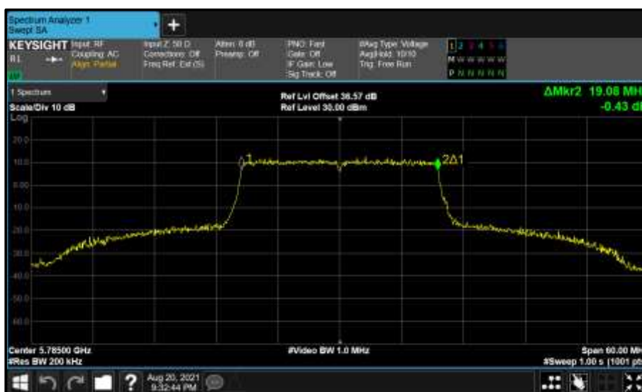
Figure 731 - Core 0 (A) 5785 MHz (CH157) 99% Bandwidth
