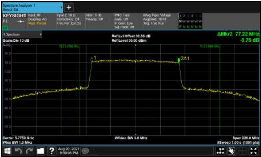
Figure 895 - Core 0 (A) 5775 MHz (CH155) 99% Bandwidth
