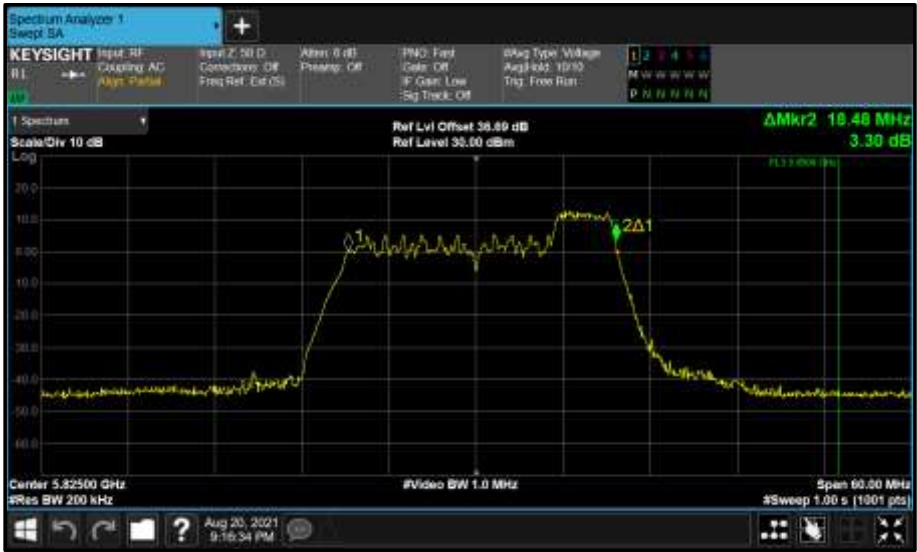
Figure 789 - Core 0 (A) 5825 MHz (CH165) 99% Bandwidth
