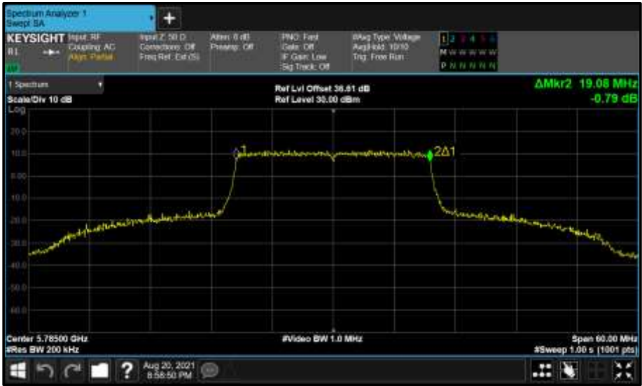
Figure 717 - Core 1 (B) 5785 MHz (CH157) 99% Bandwidth
