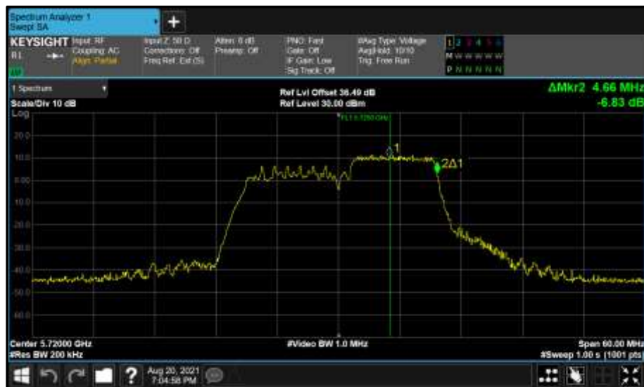
Figure 809 - Core 0 (A) 5720 MHz (CH144) 99% Bandwidth
