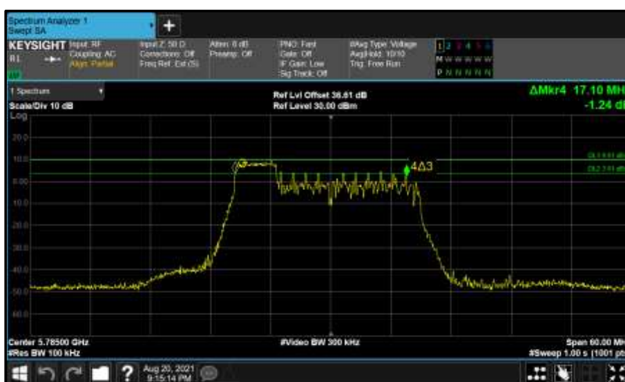
Figure 788 - Core 1 (B) 5785 MHz (CH157) 6 dB Bandwidth
