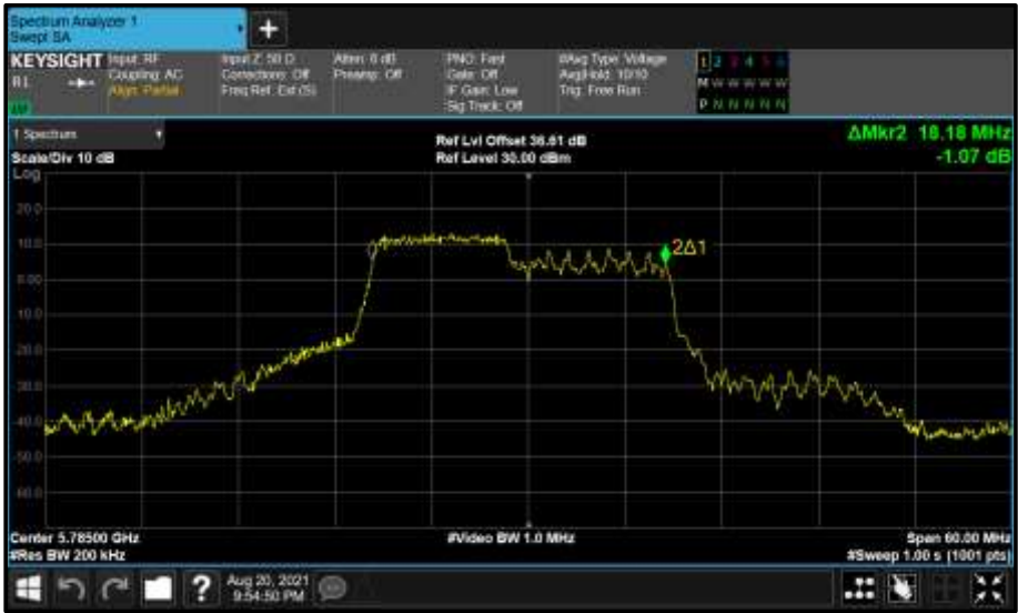
Figure 843 - Core 1 (B) 5785 MHz (CH157) 99% Bandwidth
