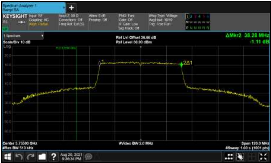
Figure 873 - Core 1 (B) 5755 MHz (CH151) 99% Bandwidth
