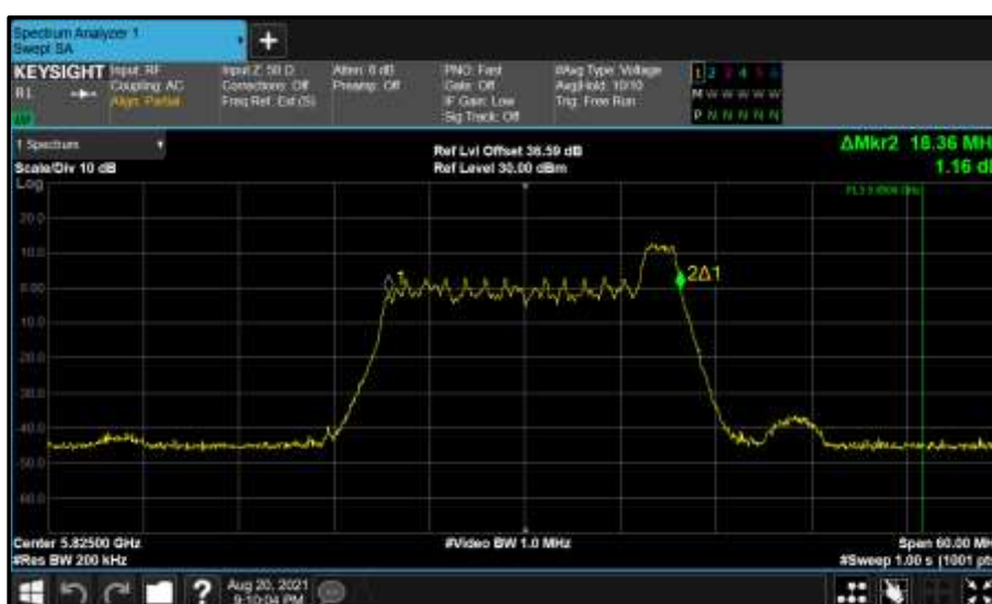
Figure 755 - Core 1 (B) 5825 MHz (CH165) 99% Bandwidth
