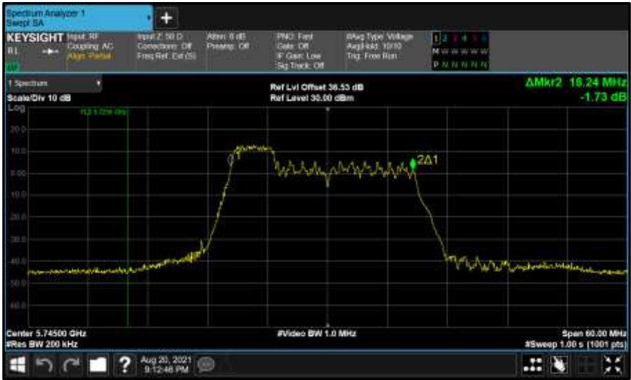
Figure 781 - Core 0 (A) 5745 MHz (CH149) 99% Bandwidth
