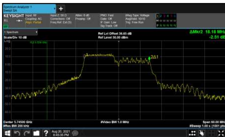
Figure 811 - Core 1 (B) 5745 MHz (CH149) 99% Bandwidth
