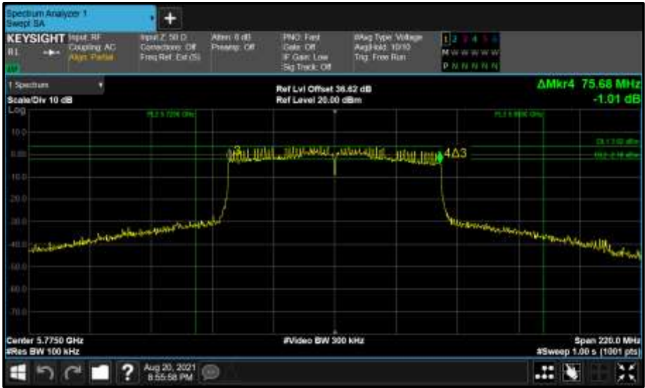
Figure 690 - Core 1 (B) 5775 MHz (CH155) 6 dB Bandwidth
