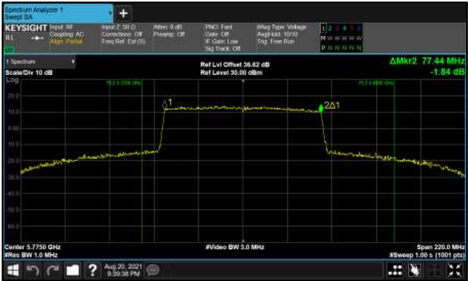
Figure 897 - Core 1 (B) 5775 MHz (CH155) 99% Bandwidth
