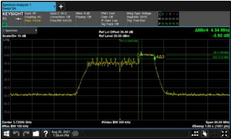
Figure 778 - Core 0 (A) 5720 MHz (CH144) 6 dB Bandwidth
