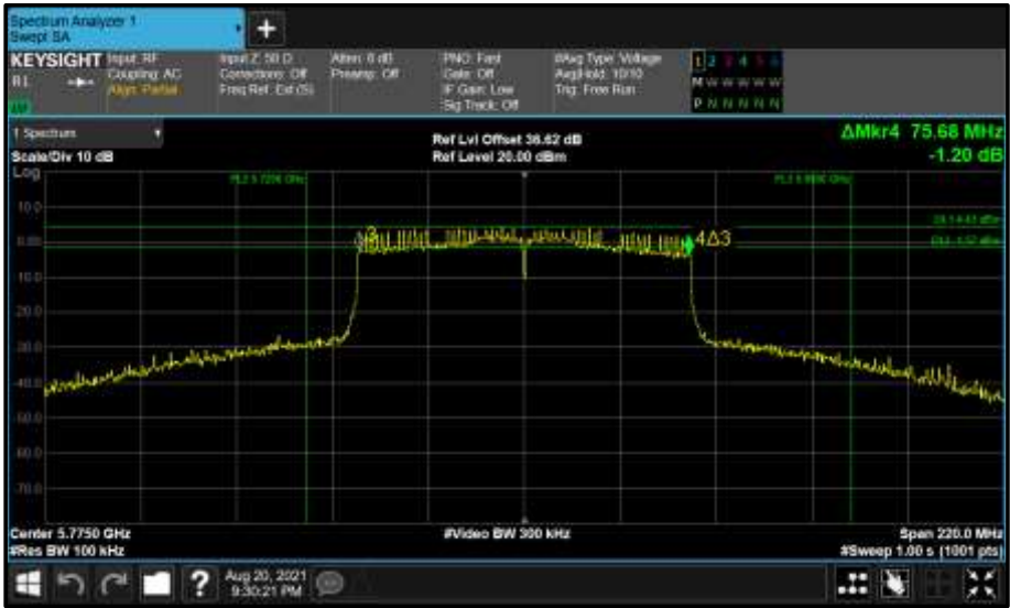
Figure 698 - Core 1 (B) 5775 MHz (CH155) 6 dB Bandwidth
