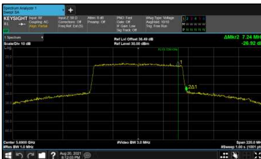
Figure 893 - Core 1 (B) 5690 MHz (CH138) 99% Bandwidth
