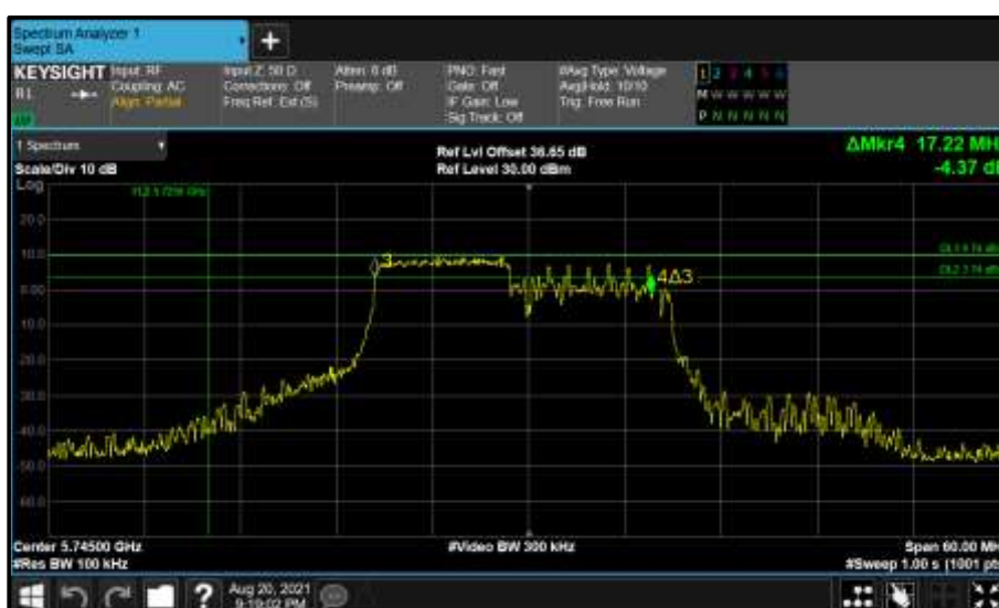
Figure 824 - Core 1 (B) 5745 MHz (CH149) 6 dB Bandwidth
