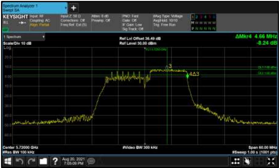
Figure 810 - Core 0 (A) 5720 MHz (CH144) 6 dB Bandwidth
