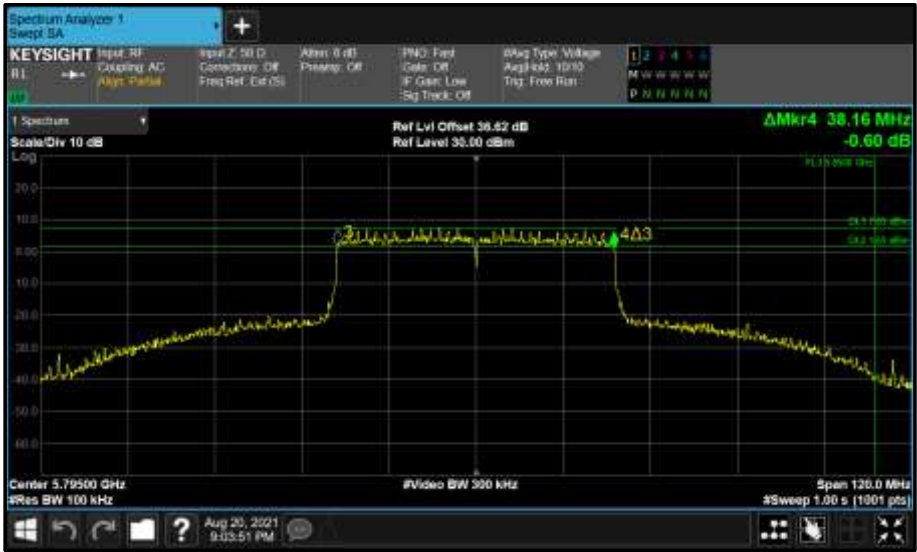
Figure 866 - Core 1 (B) 5795 MHz (CH159) 6 dB Bandwidth
