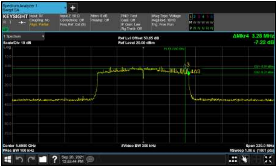
Figure 930 - Core 1 (B) 5690 MHz (CH138) 6 dB Bandwidth
