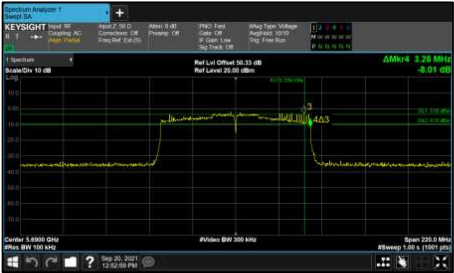
Figure 928 - Core 0 (A) 5690 MHz (CH138) 6 dB Bandwidth
