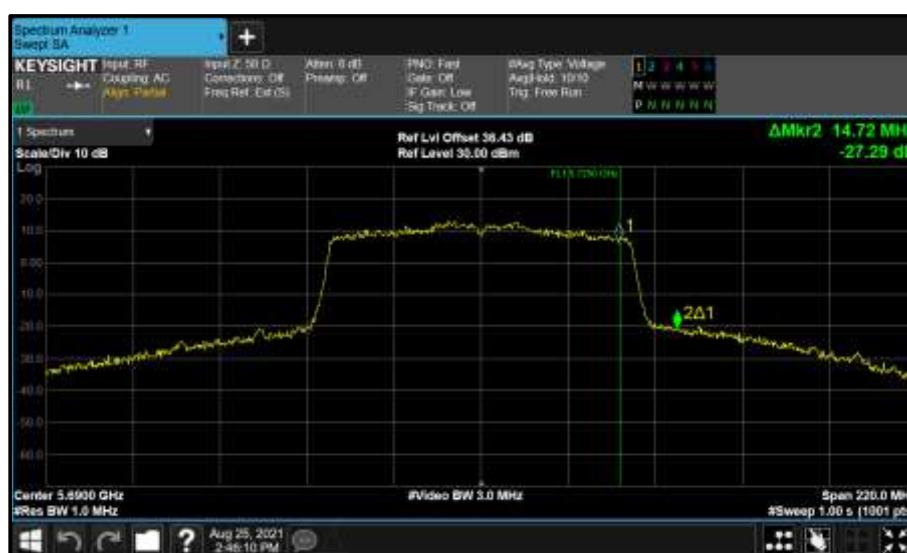
Figure 691 - Core 0 (A) 5690 MHz (CH138) 99% Bandwidth
