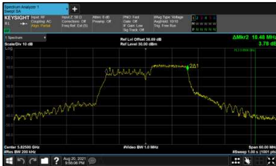
Figure 845 - Core 0 (A) 5825 MHz (CH165) 99% Bandwidth
