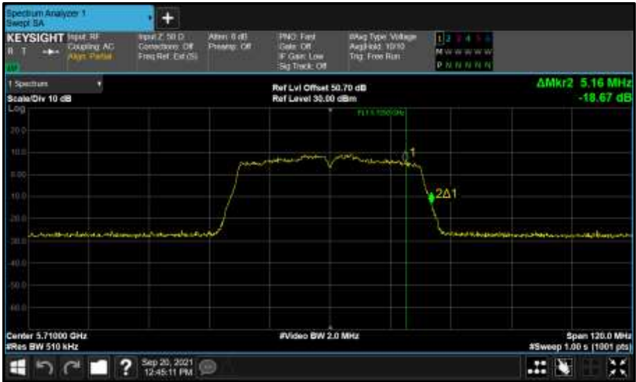
Figure 917 - Core 1 (B) 5710 MHz (CH142) 99% Bandwidth
