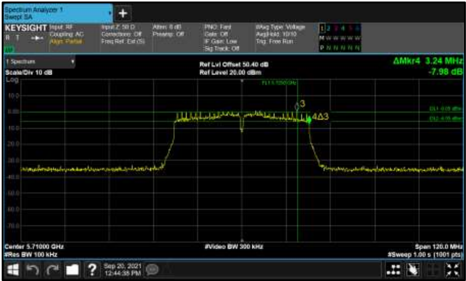
Figure 916 - Core 0 (A) 5710 MHz (CH142) 6 dB Bandwidth
