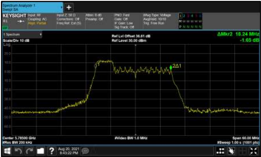
Figure 773 - Core 1 (B) 5785 MHz (CH157) 99% Bandwidth
