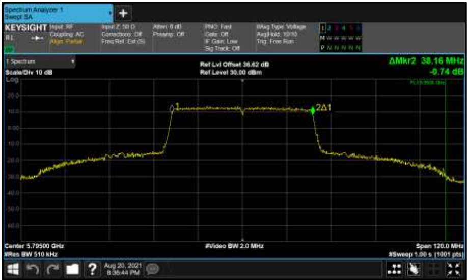
Figure 853 - Core 1 (B) 5795 MHz (CH159) 99% Bandwidth
