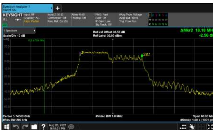
Figure 821 - Core 0 (A) 5745 MHz (CH149) 99% Bandwidth
