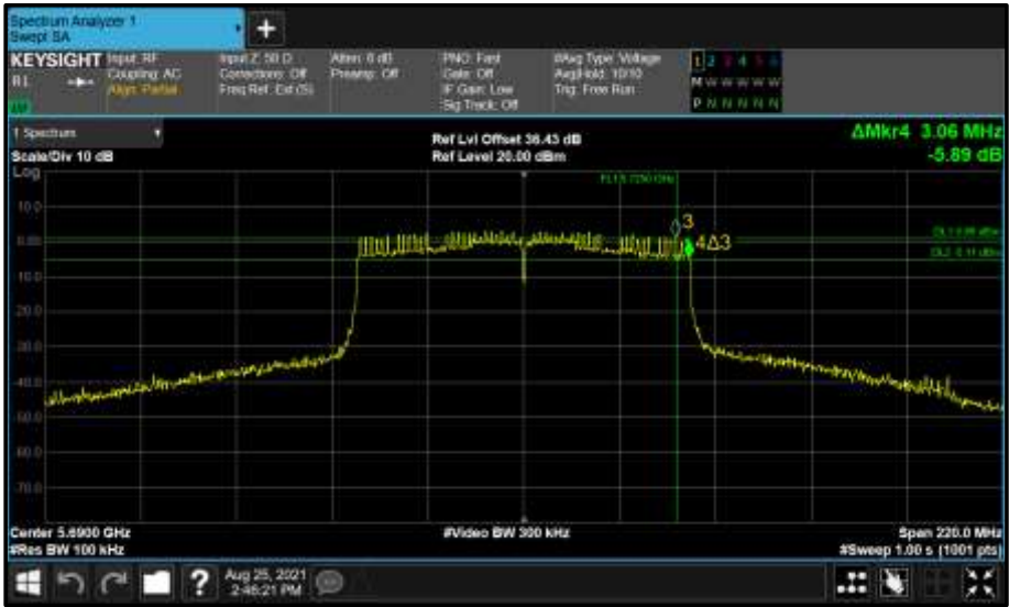
Figure 692 - Core 0 (A) 5690 MHz (CH138) 6 dB Bandwidth
