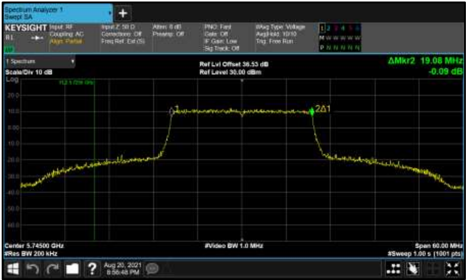
Figure 711 - Core 0 (A) 5745 MHz (CH149) 99% Bandwidth
