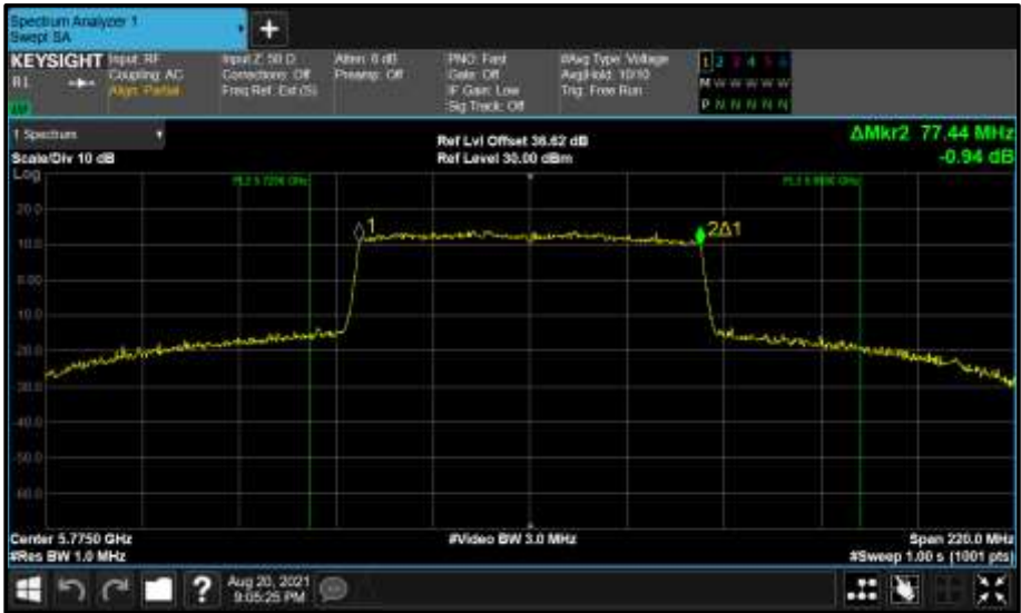
Figure 889 - Core 1 (B) 5775 MHz (CH155) 99% Bandwidth
