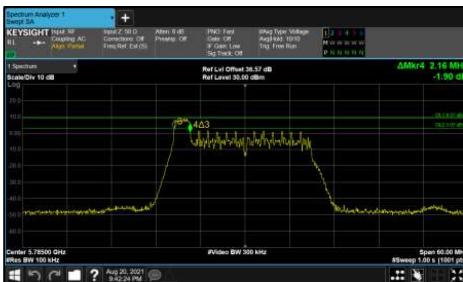
Figure 762 - Core 0 (A) 5785 MHz (CH157) 6 dB Bandwidth
