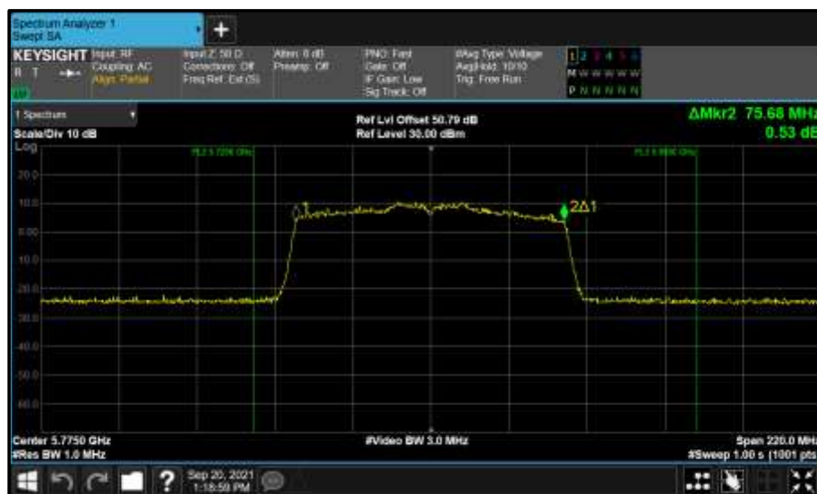
Figure 933 - Core 1 (B) 5775 MHz (CH155) 99% Bandwidth
