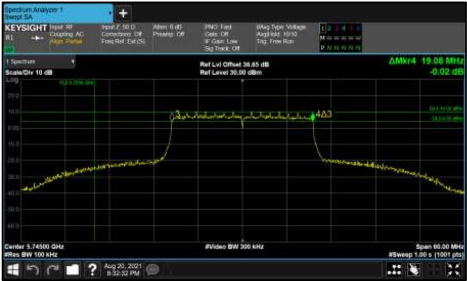
Figure 702 - Core 1 (B) 5745 MHz (CH149) 6 dB Bandwidth
