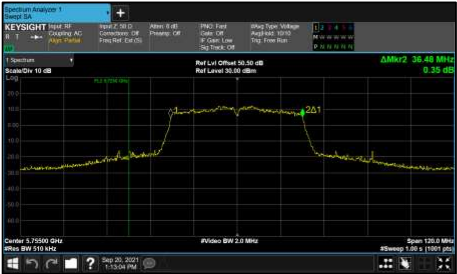
Figure 919 - Core 0 (A) 5755 MHz (CH151) 99% Bandwidth
