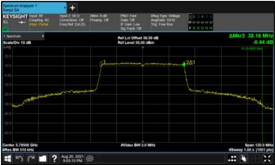
Figure 863 - Core 0 (A) 5795 MHz (CH159) 99% Bandwidth
