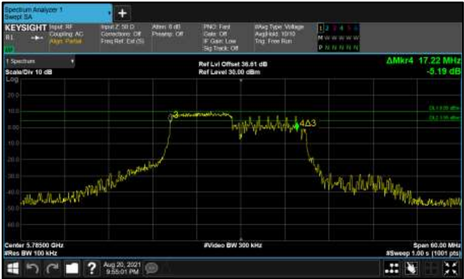
Figure 844 - Core 1 (B) 5785 MHz (CH157) 6 dB Bandwidth
