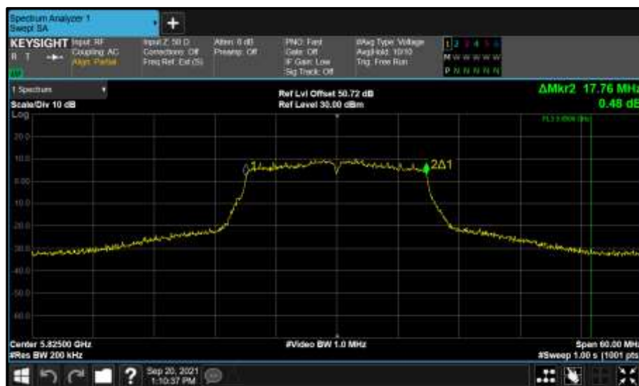
Figure 911 - Core 0 (A) 5825 MHz (CH165) 99% Bandwidth
