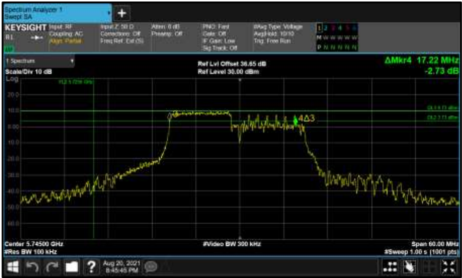
Figure 812 - Core 1 (B) 5745 MHz (CH149) 6 dB Bandwidth
