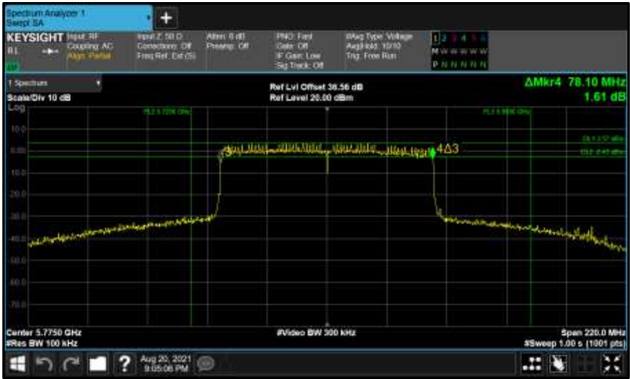
Figure 888 - Core 0 (A) 5775 MHz (CH155) 6 dB Bandwidth
