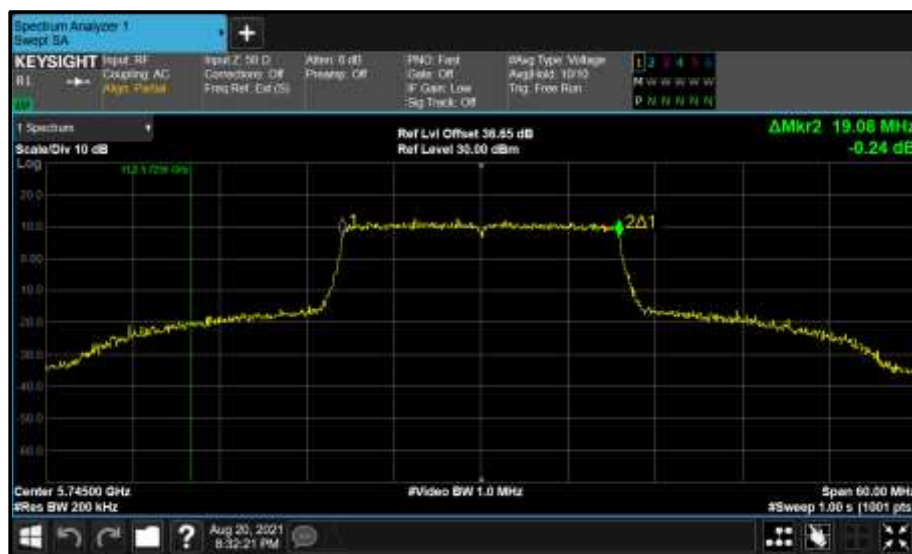
Figure 701 - Core 1 (B) 5745 MHz (CH149) 99% Bandwidth
