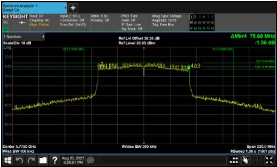
Figure 696 - Core 0 (A) 5775 MHz (CH155) 6 dB Bandwidth
