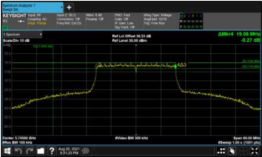
Figure 728 - Core 0 (A) 5745 MHz (CH149) 6 dB Bandwidth
