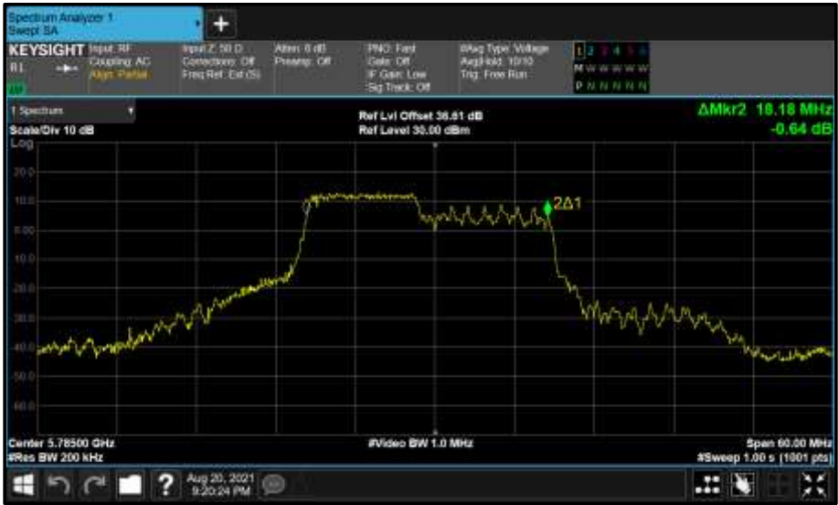
Figure 827 - Core 1 (B) 5785 MHz (CH157) 99% Bandwidth
