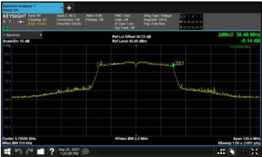
Figure 923 - Core 0 (A) 5795 MHz (CH159) 99% Bandwidth
