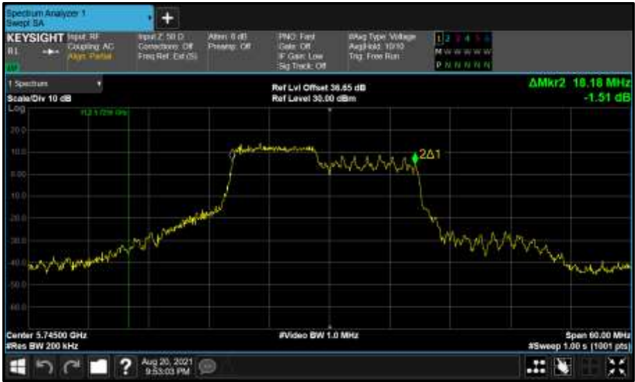
Figure 839 - Core 1 (B) 5745 MHz (CH149) 99% Bandwidth
