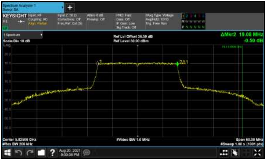
Figure 721 - Core 1 (B) 5825 MHz (CH165) 99% Bandwidth
