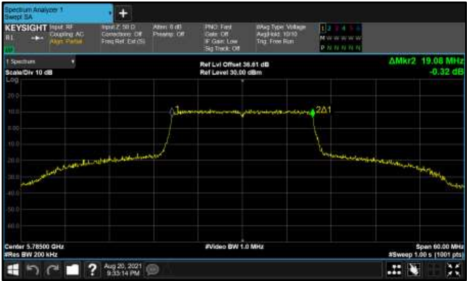
Figure 733 - Core 1 (B) 5785 MHz (CH157) 99% Bandwidth
