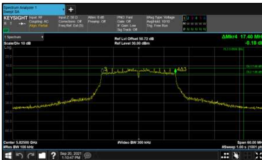
Figure 912 - Core 0 (A) 5825 MHz (CH165) 6 dB Bandwidth
