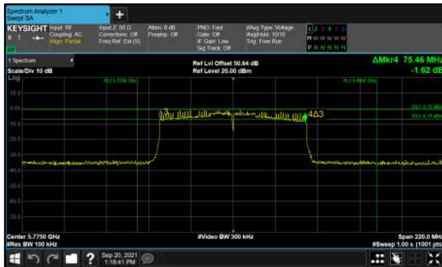
Figure 932 - Core 0 (A) 5775 MHz (CH155) 6 dB Bandwidth
