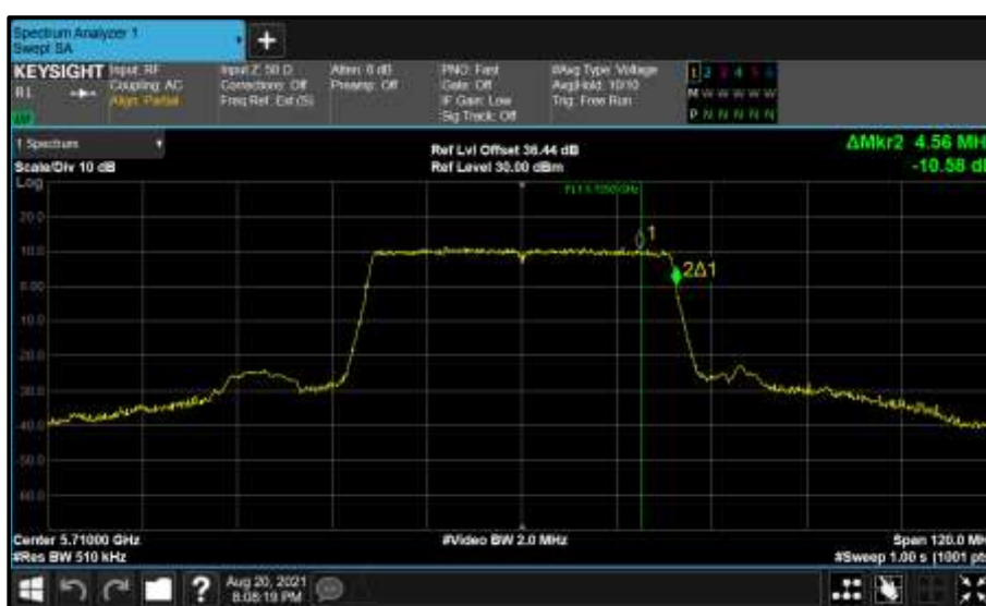
Figure 867 - Core 0 (A) 5710 MHz (CH142) 99% Bandwidth
