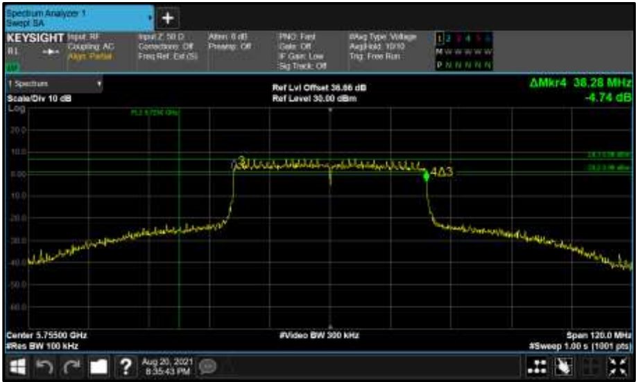
Figure 852 - Core 1 (B) 5755 MHz (CH151) 6 dB Bandwidth
