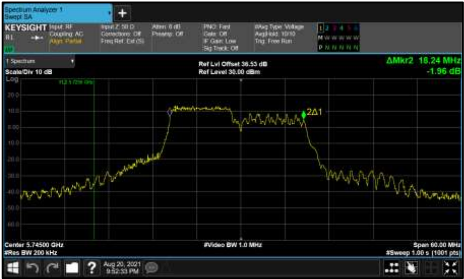
Figure 837 - Core 0 (A) 5745 MHz (CH149) 99% Bandwidth
