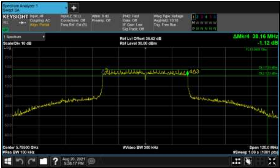
Figure 878 - Core 1 (B) 5795 MHz (CH159) 6 dB Bandwidth
