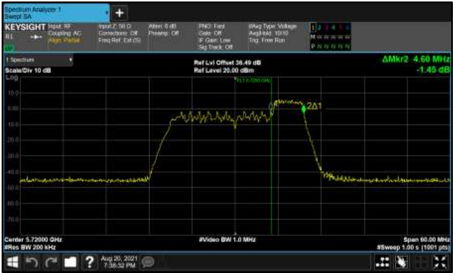
Figure 777 - Core 0 (A) 5720 MHz (CH144) 99% Bandwidth
