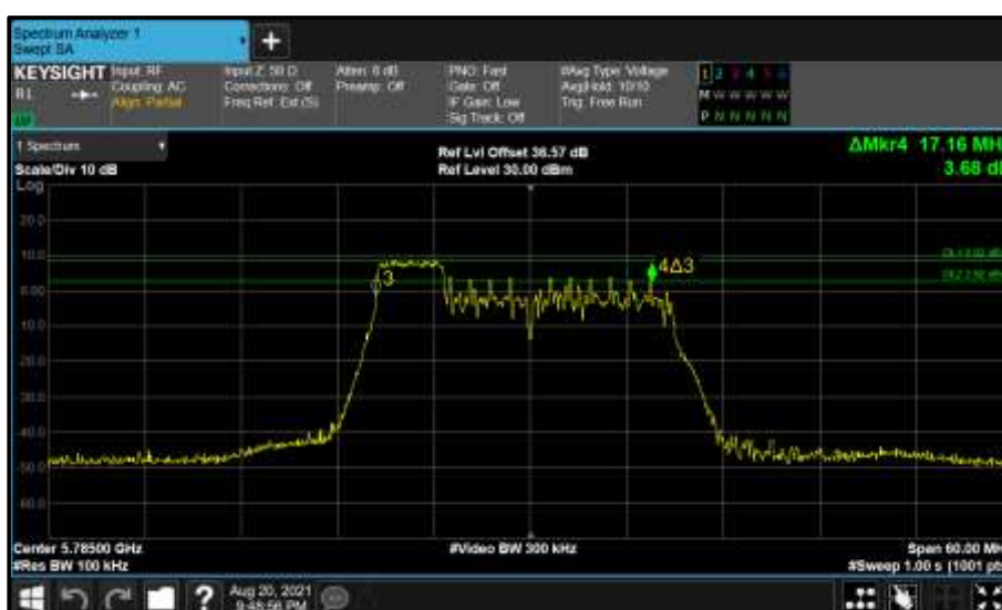
Figure 802 - Core 0 (A) 5785 MHz (CH157) 6 dB Bandwidth
