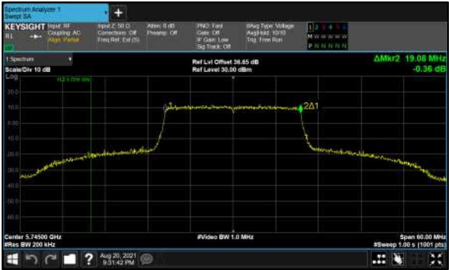
Figure 729 - Core 1 (B) 5745 MHz (CH149) 99% Bandwidth
