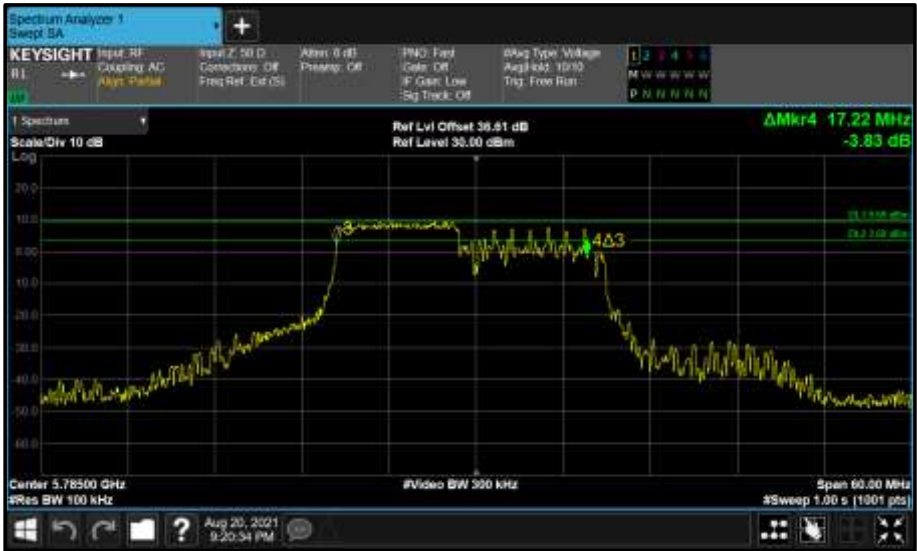
Figure 828 - Core 1 (B) 5785 MHz (CH157) 6 dB Bandwidth
