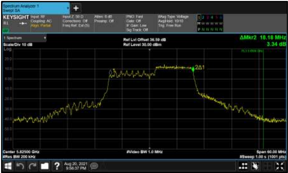
Figure 847 - Core 1 (B) 5825 MHz (CH165) 99% Bandwidth
