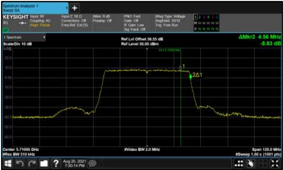
Figure 857 - Core 1 (B) 5710 MHz (CH142) 99% Bandwidth
