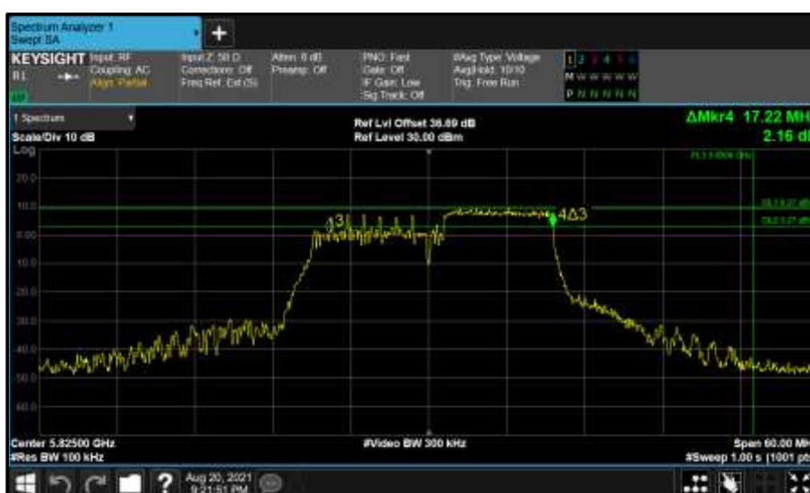
Figure 830 - Core 0 (A) 5825 MHz (CH165) 6 dB Bandwidth
