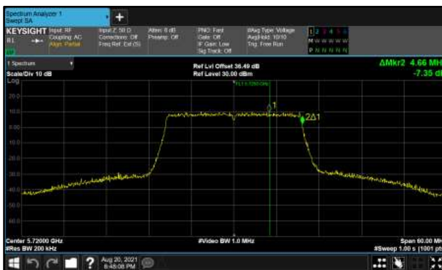
Figure 699 - Core 0 (A) 5720 MHz (CH144) 99% Bandwidth
