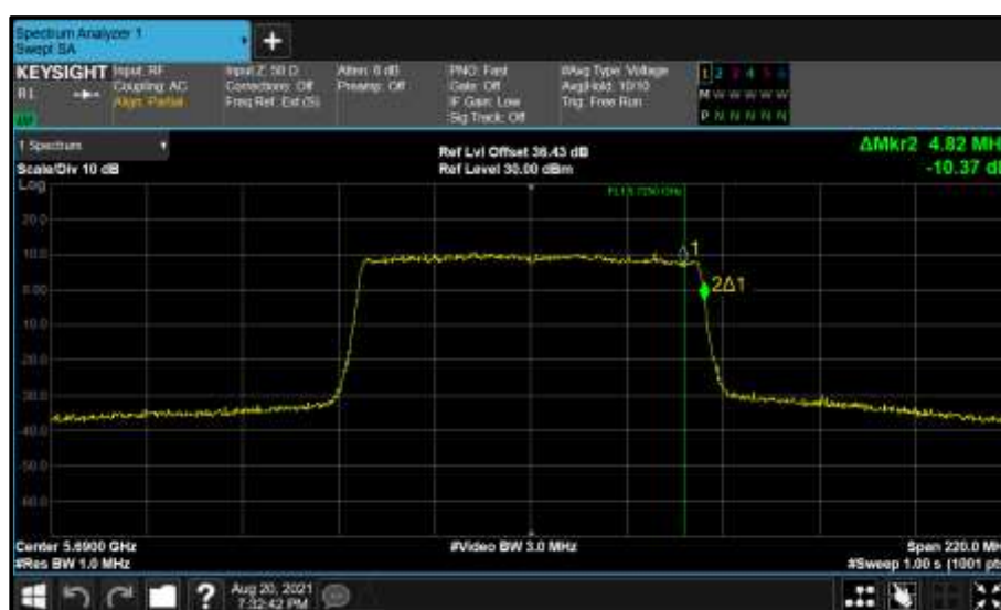
Figure 883 - Core 0 (A) 5690 MHz (CH138) 99% Bandwidth
