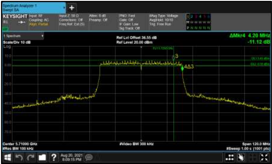
Figure 870 - Core 1 (B) 5710 MHz (CH142) 6 dB Bandwidth
