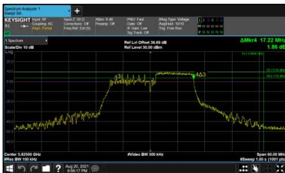
Figure 846 - Core 0 (A) 5825 MHz (CH165) 6 dB Bandwidth
