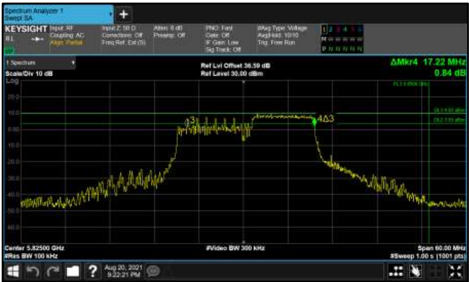
Figure 832 - Core 1 (B) 5825 MHz (CH165) 6 dB Bandwidth
