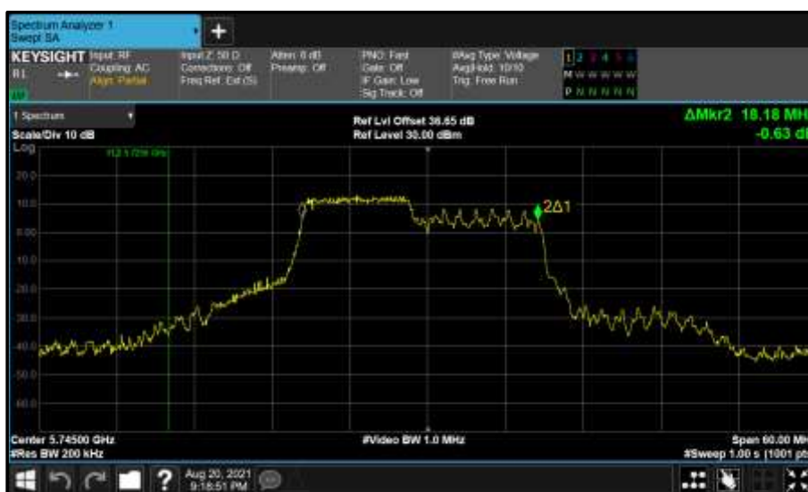
Figure 823 - Core 1 (B) 5745 MHz (CH149) 99% Bandwidth
