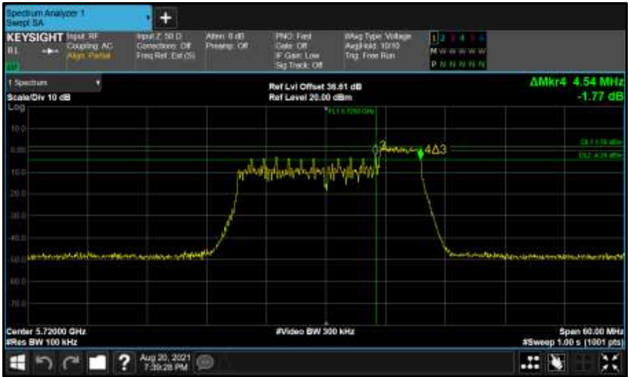
Figure 780 - Core 1 (B) 5720 MHz (CH144) 6 dB Bandwidth
