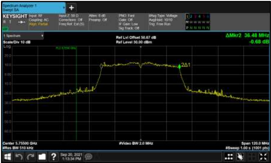
Figure 921 - Core 1 (B) 5755 MHz (CH151) 99% Bandwidth
