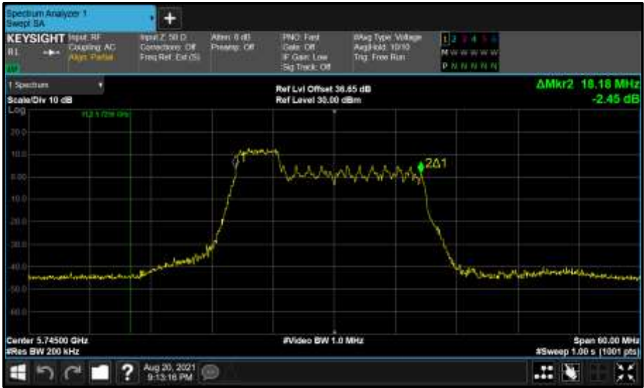
Figure 783 - Core 1 (B) 5745 MHz (CH149) 99% Bandwidth
