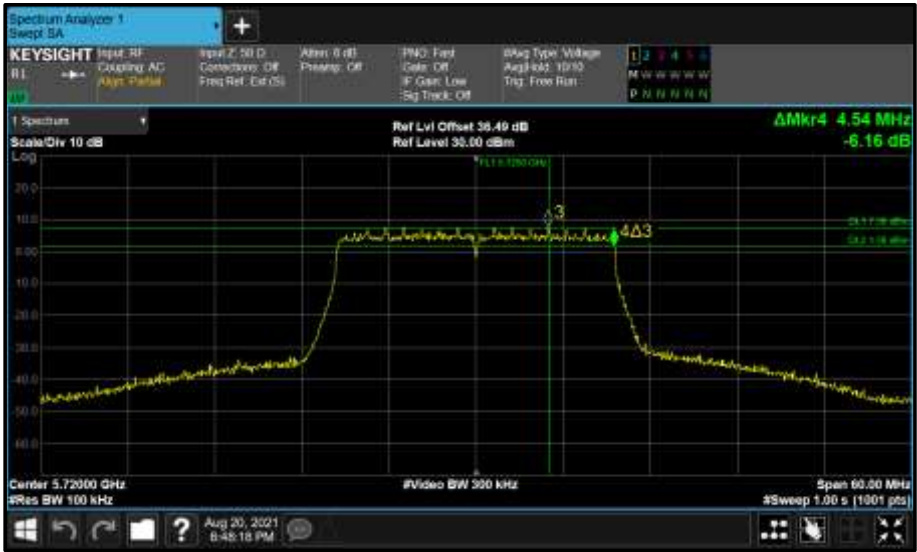
Figure 700 - Core 0 (A) 5720 MHz (CH144) 6 dB Bandwidth
