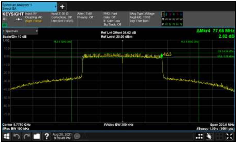
Figure 898 - Core 1 (B) 5775 MHz (CH155) 6 dB Bandwidth
