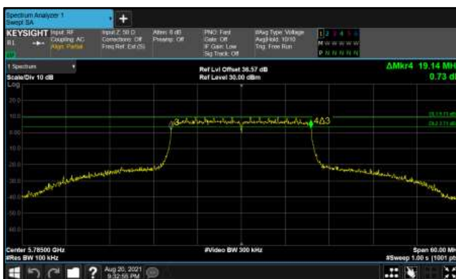
Figure 732 - Core 0 (A) 5785 MHz (CH157) 6 dB Bandwidth
