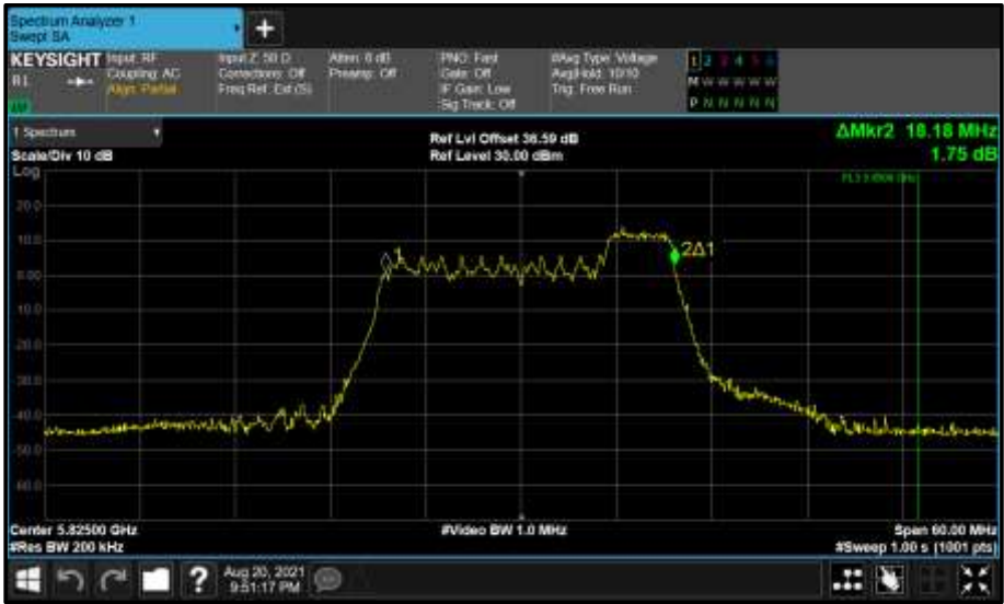
Figure 807 - Core 1 (B) 5825 MHz (CH165) 99% Bandwidth
