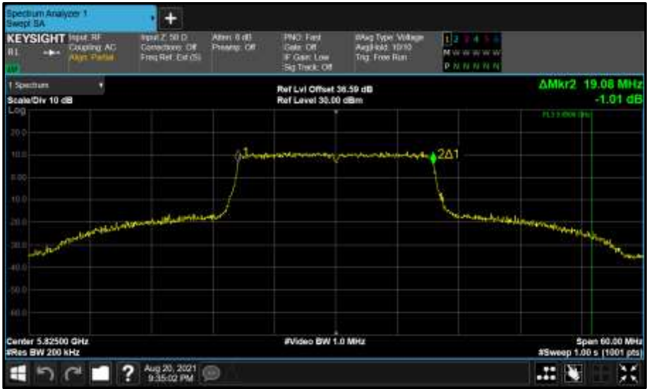
Figure 737 - Core 1 (B) 5825 MHz (CH165) 99% Bandwidth
