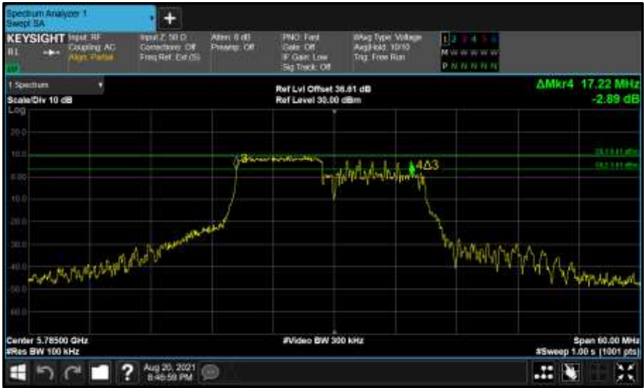
Figure 814 - Core 1 (B) 5785 MHz (CH157) 6 dB Bandwidth
