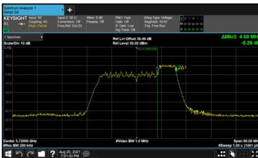
Figure 769 - Core 0 (A) 5720 MHz (CH144) 99% Bandwidth
