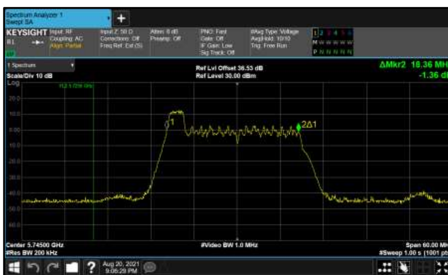
Figure 745 - Core 0 (A) 5745 MHz (CH149) 99% Bandwidth
