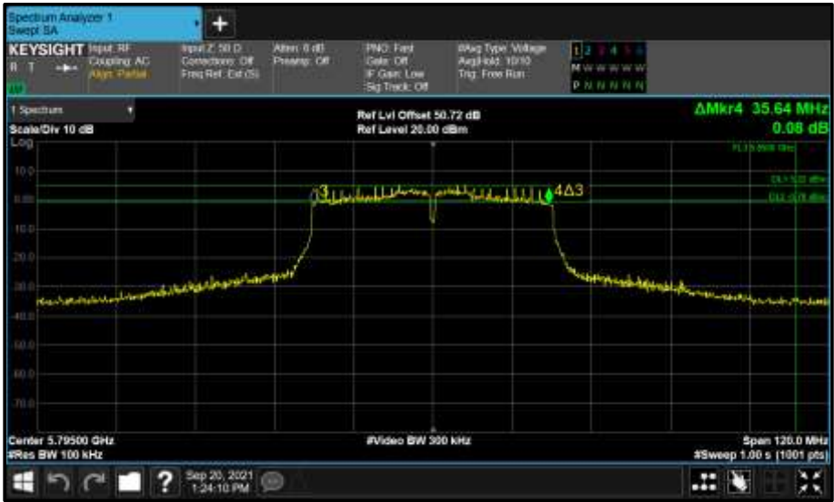
Figure 924 - Core 0 (A) 5795 MHz (CH159) 6 dB Bandwidth
