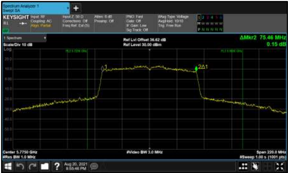
Figure 689 - Core 1 (B) 5775 MHz (CH155) 99% Bandwidth
