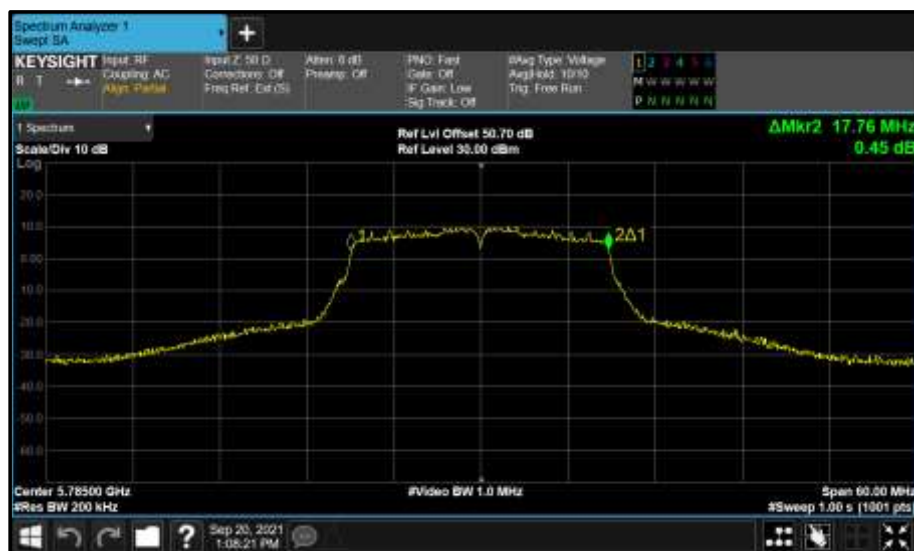
Figure 907 - Core 0 (A) 5785 MHz (CH157) 99% Bandwidth
