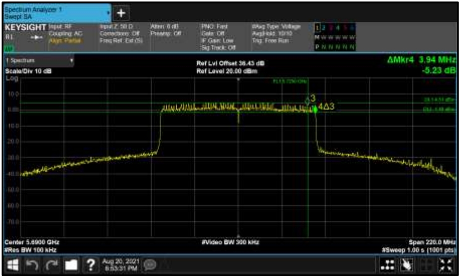
Figure 880 - Core 0 (A) 5690 MHz (CH138) 6 dB Bandwidth
