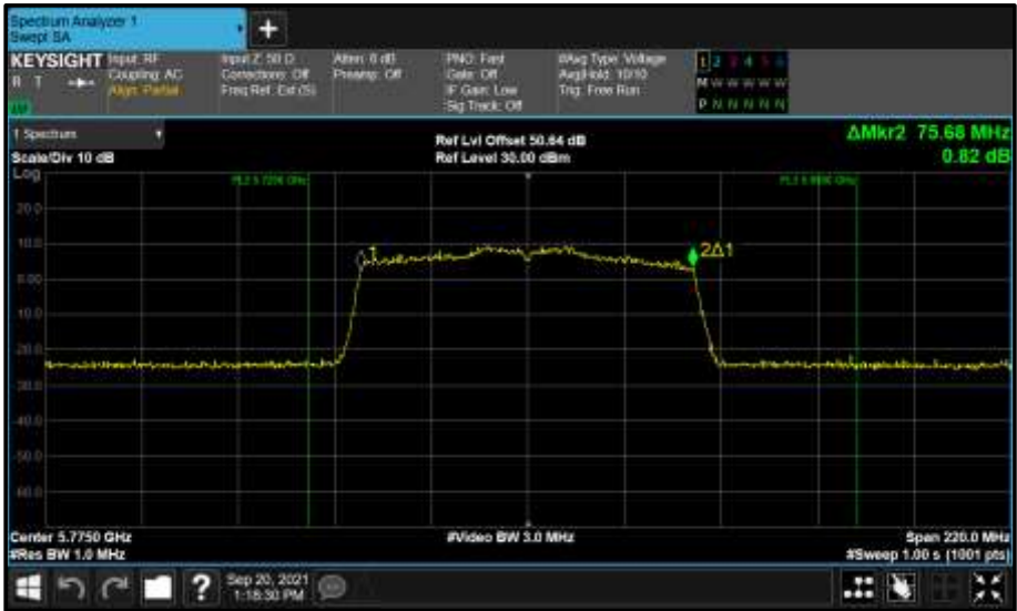
Figure 931 - Core 0 (A) 5775 MHz (CH155) 99% Bandwidth
