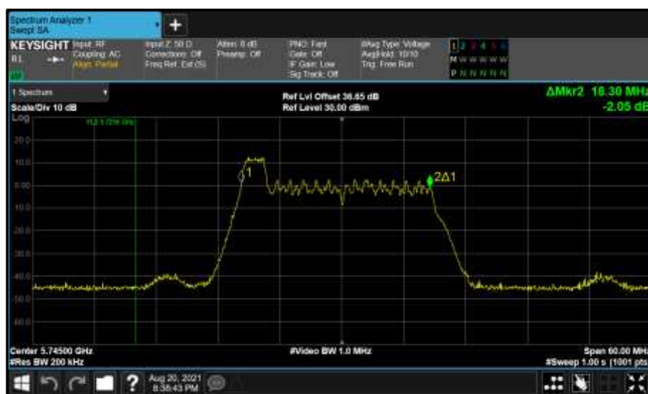
Figure 739 - Core 1 (B) 5745 MHz (CH149) 99% Bandwidth
