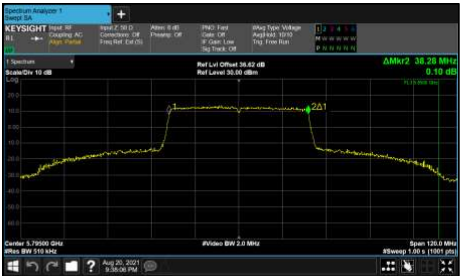
Figure 877 - Core 1 (B) 5795 MHz (CH159) 99% Bandwidth
