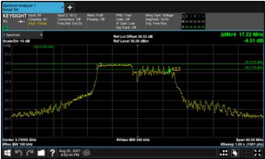
Figure 838 - Core 0 (A) 5745 MHz (CH149) 6 dB Bandwidth
