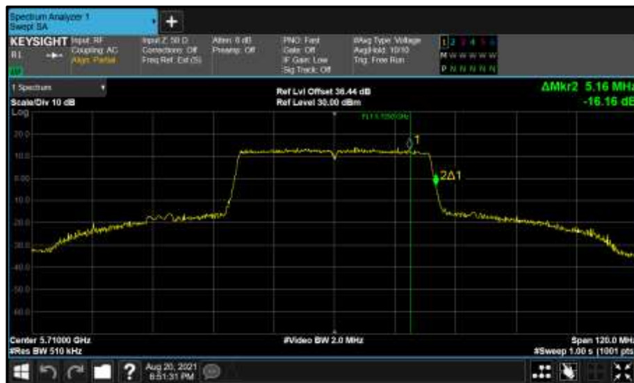
Figure 849 - Core 0 (A) 5710 MHz (CH142) 99% Bandwidth
