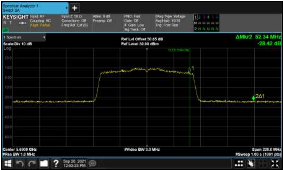
Figure 929 - Core 1 (B) 5690 MHz (CH138) 99% Bandwidth
