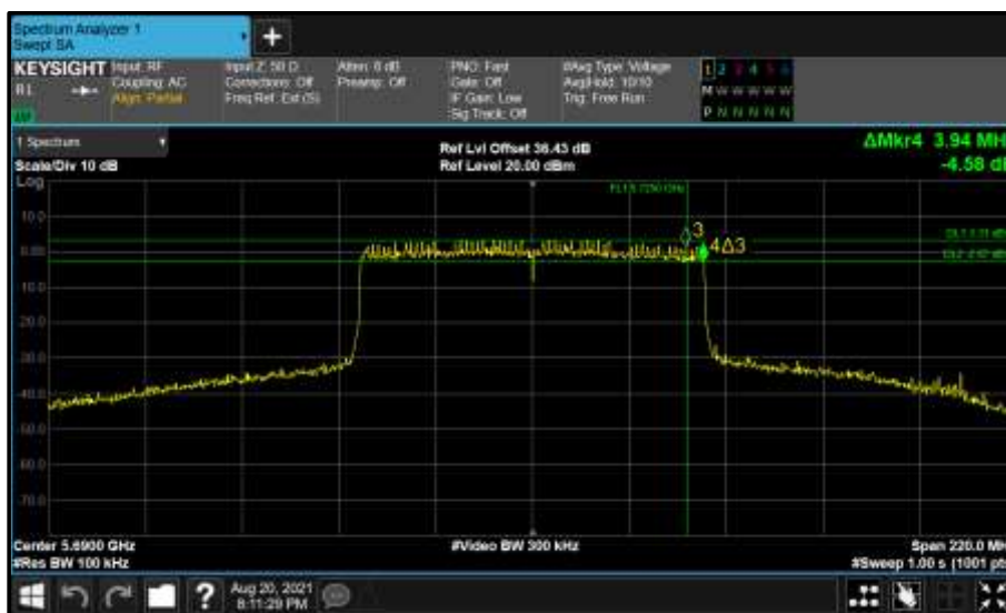
Figure 892 - Core 0 (A) 5690 MHz (CH138) 6 dB Bandwidth
