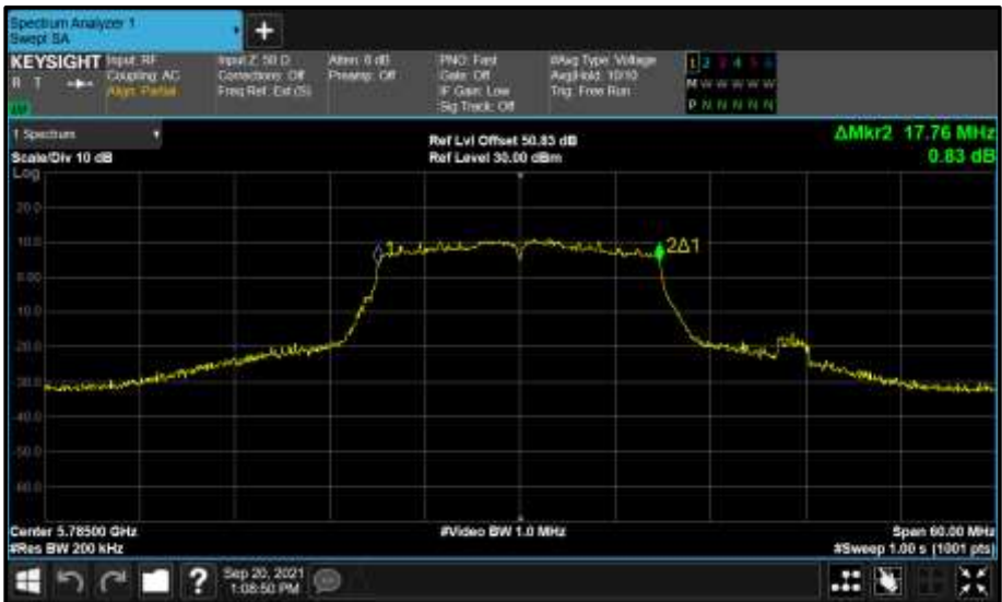
Figure 909 - Core 1 (B) 5785 MHz (CH157) 99% Bandwidth
