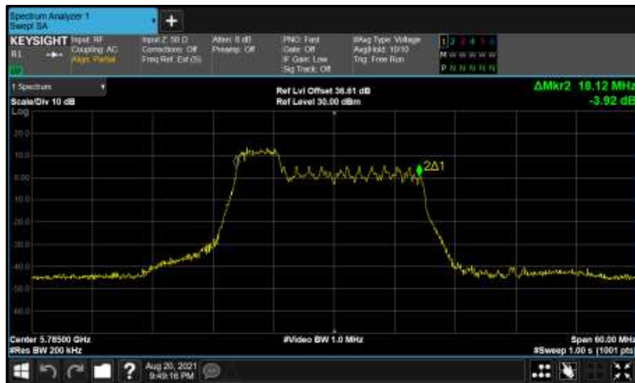
Figure 803 - Core 1 (B) 5785 MHz (CH157) 99% Bandwidth
