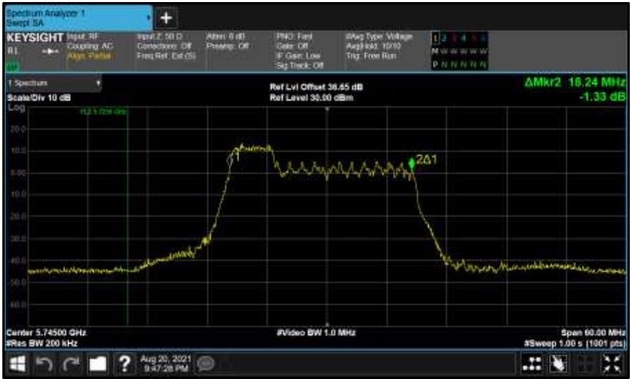
Figure 799 - Core 1 (B) 5745 MHz (CH149) 99% Bandwidth
