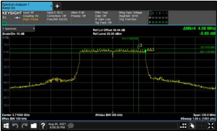
Figure 868 - Core 0 (A) 5710 MHz (CH142) 6 dB Bandwidth
