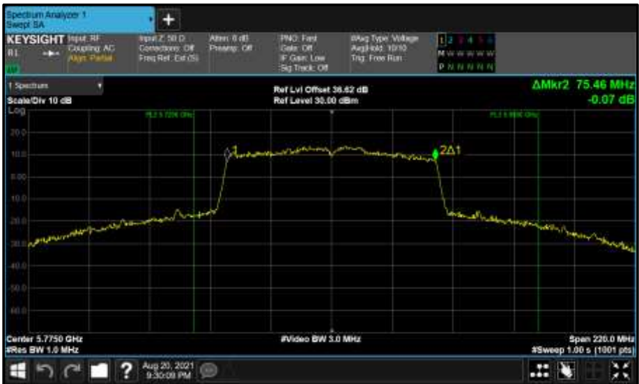
Figure 697 - Core 1 (B) 5775 MHz (CH155) 99% Bandwidth
