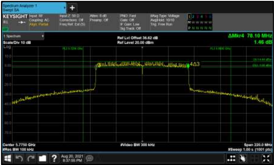
Figure 882 - Core 1 (B) 5775 MHz (CH155) 6 dB Bandwidth
