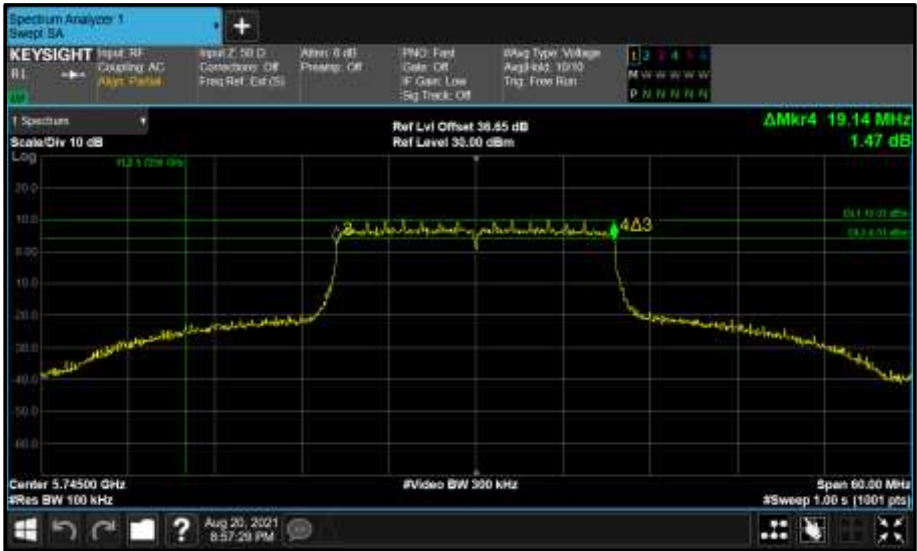
Figure 714 - Core 1 (B) 5745 MHz (CH149) 6 dB Bandwidth
