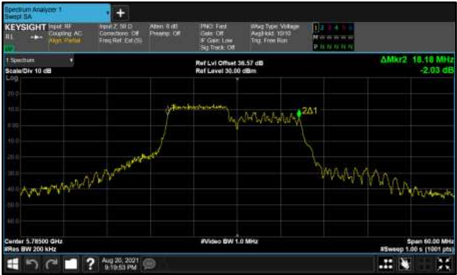
Figure 825 - Core 0 (A) 5785 MHz (CH157) 99% Bandwidth
