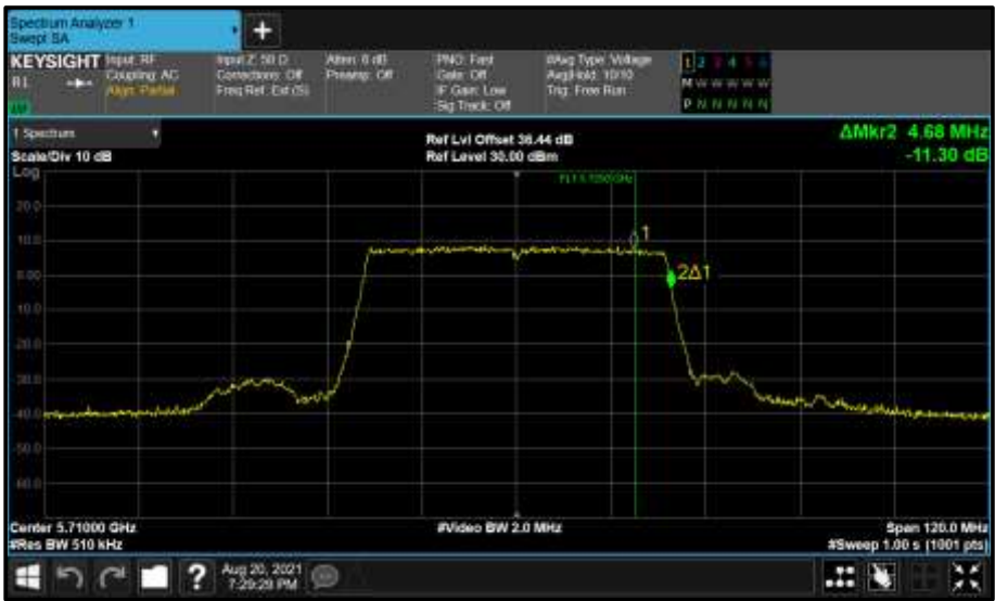
Figure 855 - Core 0 (A) 5710 MHz (CH142) 99% Bandwidth
