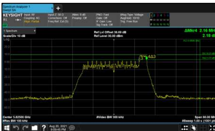
Figure 754 - Core 0 (A) 5825 MHz (CH165) 6 dB Bandwidth
