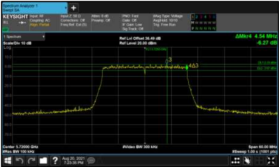
Figure 708 - Core 0 (A) 5720 MHz (CH144) 6 dB Bandwidth
