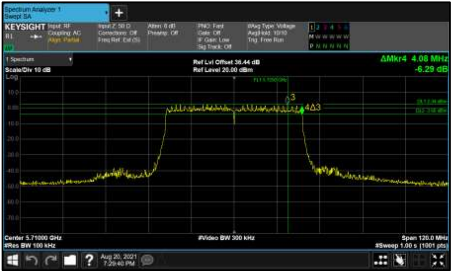
Figure 856 - Core 0 (A) 5710 MHz (CH142) 6 dB Bandwidth
