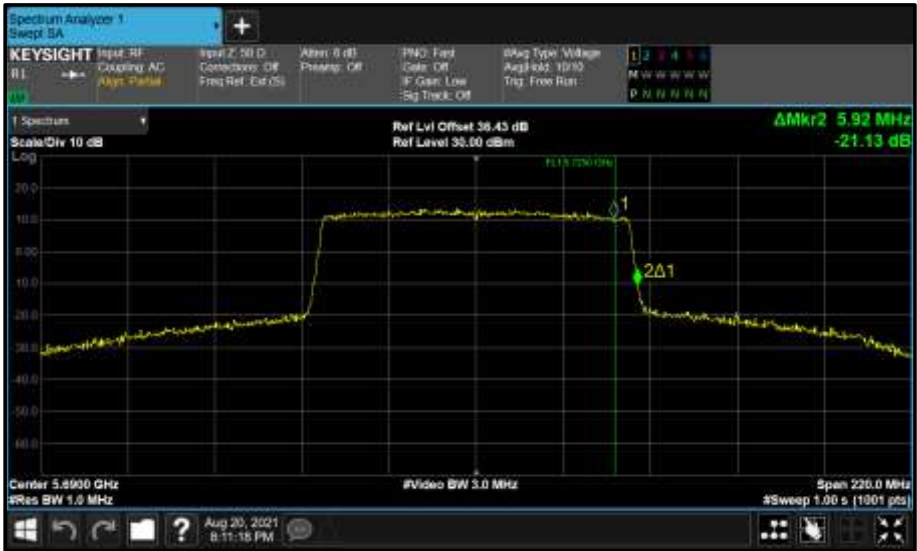
Figure 891 - Core 0 (A) 5690 MHz (CH138) 99% Bandwidth
