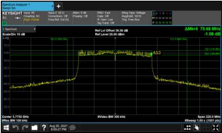
Figure 688 - Core 0 (A) 5775 MHz (CH155) 6 dB Bandwidth
