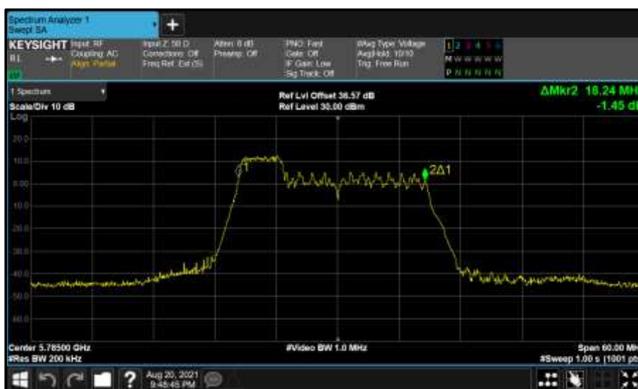
Figure 801 - Core 0 (A) 5785 MHz (CH157) 99% Bandwidth
