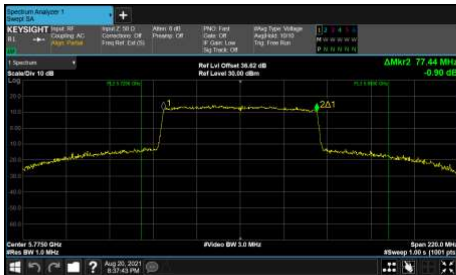
Figure 881 - Core 1 (B) 5775 MHz (CH155) 99% Bandwidth
