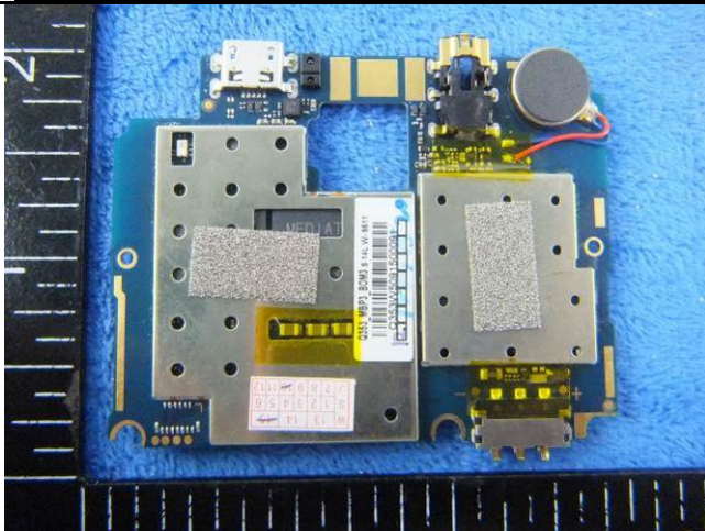
Mainboard with Shielding - Rear View
