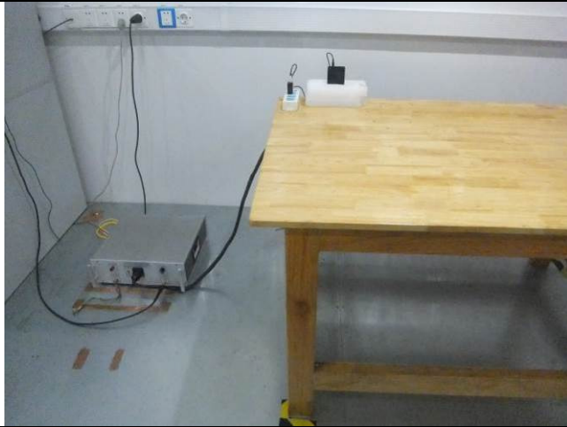
Conducted Emissions Test Setup Front View
