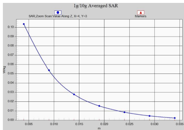
Fig. 1-11 Z-Scan at power reference point (LTE Band 41)
