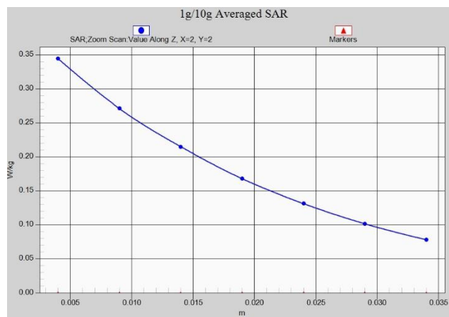
Fig. 1-2 Z-Scan at power reference point (GSM850)
